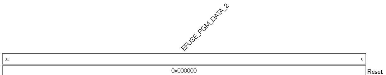
Register 5.3. EFUSE_PGM_DATA2_REG (0x0008)
