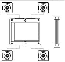
Pico4ML-Pro can also work as a multiple SPI camera adapter. Up to 4 Arducam Mega SPI cameras can be connected to the Pico4ML-Pro simultaneously.
