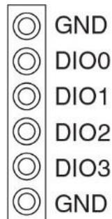
Figure 4. Screw terminal pinout.
