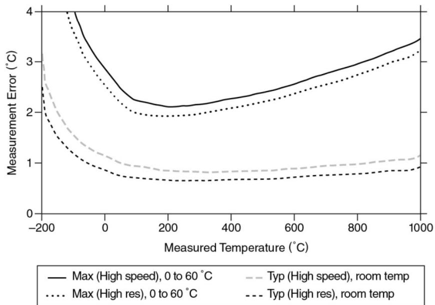
Thermocouple Type T and E Errors
