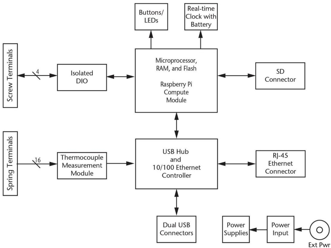
Figure 2. WebDAQ 316 functional block diagram
