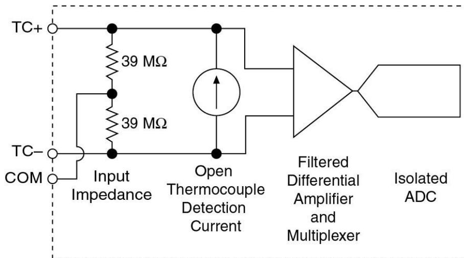
Figure 7. Input circuitry of one TC channel
