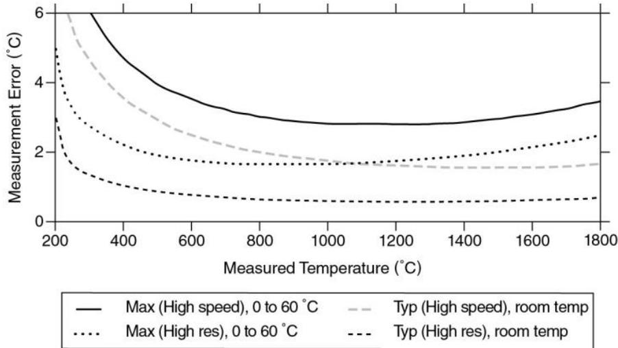
Thermocouple Type B Errors
