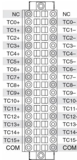
Figure 5. Spring terminal pinout.
