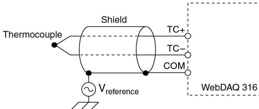
Figure 6. Typical thermocouple connection
