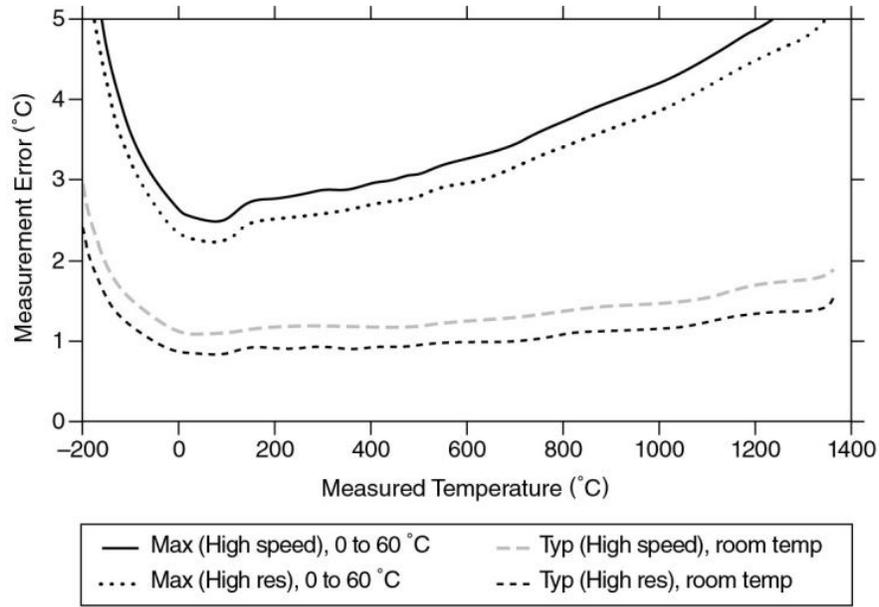
Thermocouple Type K Errors
