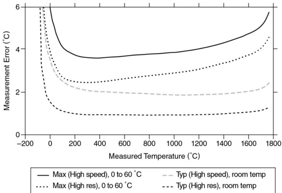
Thermocouple Type R and S Errors
