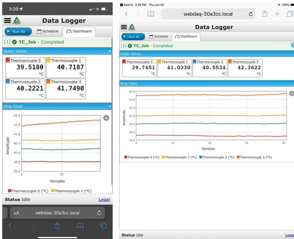
*Device-independent operation lets you remotely monitor and control the WebDAQ 316 from any device with a web browser.*
