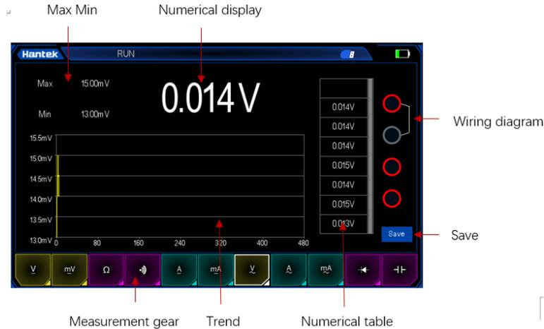
Figure 16.1 Multimeter
