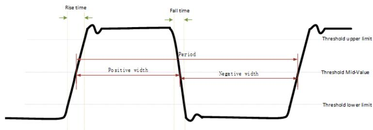
1. Period: Defined as the time between the mid-threshold intersection of two continuous, homopolar edges.
