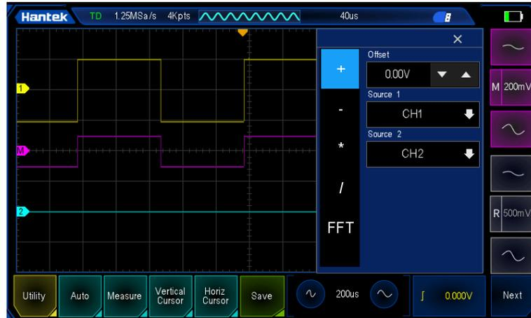
Figure 7.2 Addition operation
