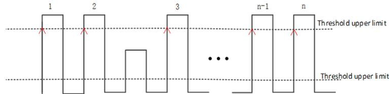
4. Number of falling edges: The number of falling edges falling from above the upper threshold to below the lower threshold.
