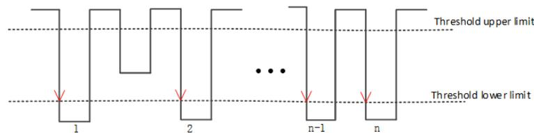
5. Trigger count: The number of rising edges (or falling edges).
