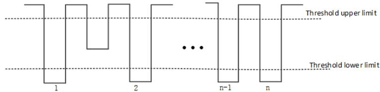
3. Number of rising edges: The number of rising edges rising from below the lower threshold to above the upper threshold.
