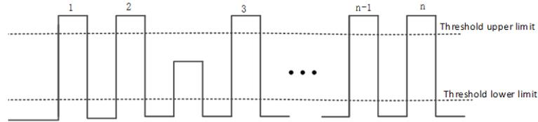
2. Number of negative pulses: The number of negative pulses falling from above the upper threshold to below the lower threshold.
