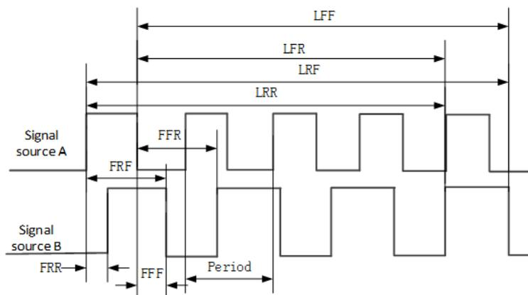
Data sources A and B, i.e., data sources A and B in the measurement settings menu, can be any channel in CH1- CH4.
