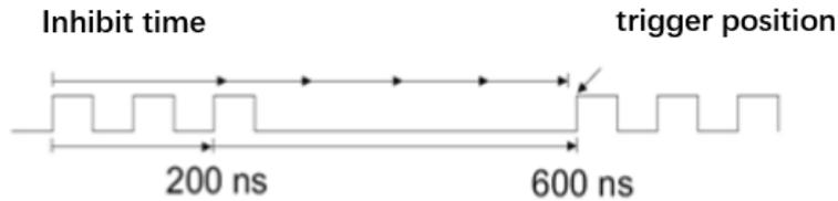
Figure 9.1 Trigger hold-off
