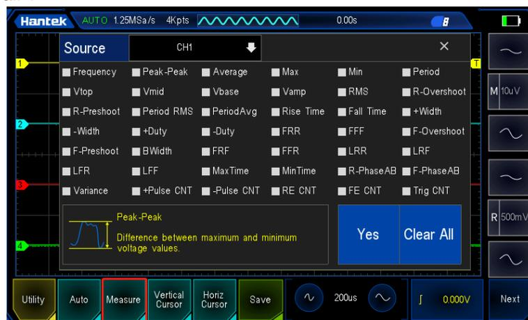
Figure 10.1 Measurement parameters
