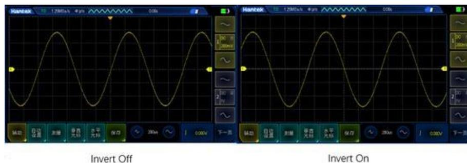
Figure 6.2 Waveform inversion
