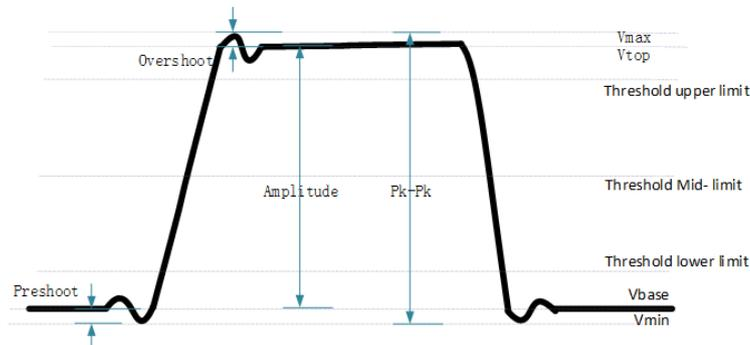
1. [Vmax] : voltage from the highest point of the waveform to GND.
