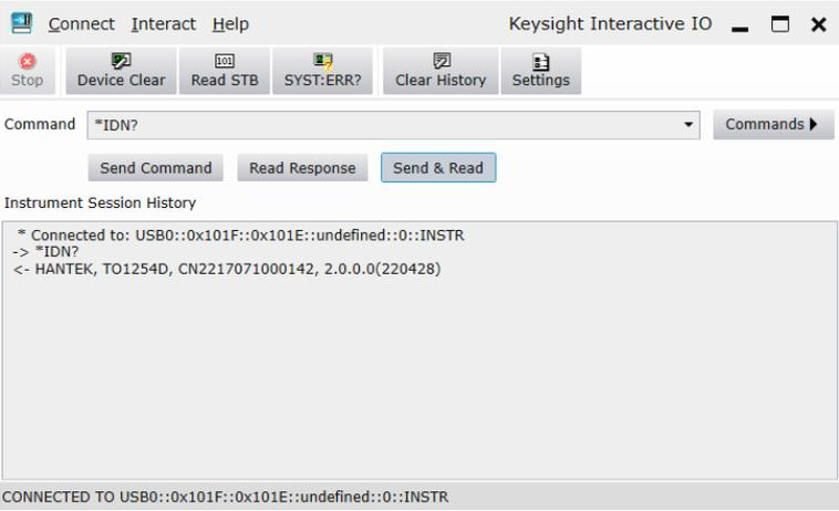
Double-click to open the upper computer software. If you see the connection information in the lower left corner of the interface, it indicates the upper computer has been connected.
