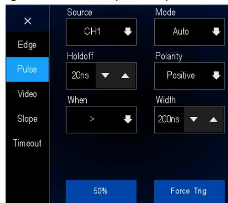
Figure 9.3 Pulse width trigger menu
