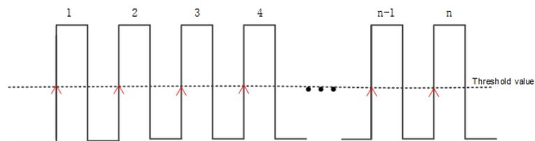
**Note:** The above measurements only apply to analog channels. The upper and lower thresholds are 90% and 10% respectively.
