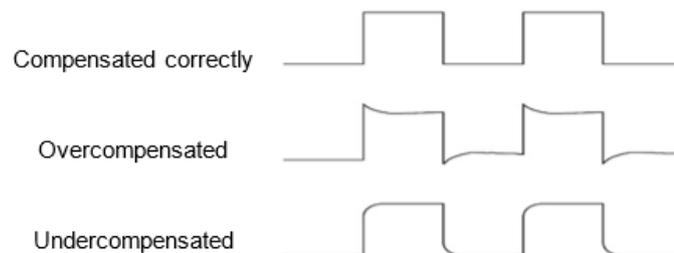
Figure 4.4 Probe compensation4
