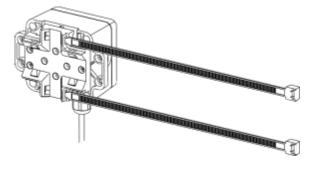
(3) To lock the device to the pole:
