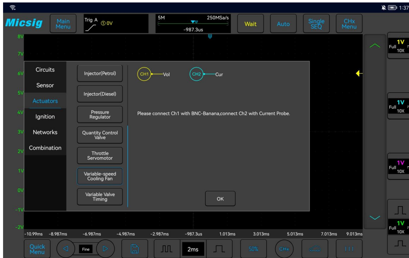
Figure 3-40 Variable-speed Cooling fan test
