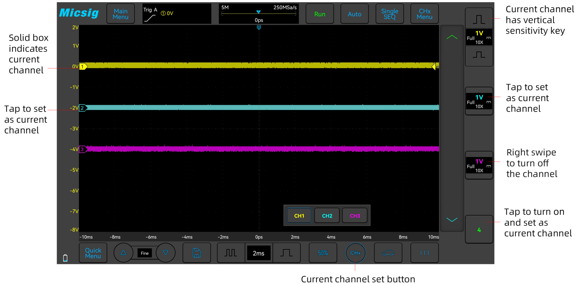
Figure 5-4 Channel Open, Close and Switching
