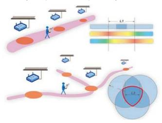
Deployment strategies vary across scenarios. For instance, indoor settings might involve central (narrow) placement or triangular grid distribution (sparse). In indoor corridors, options include centerline deployment (for corridors around 3m wide) or dual-column arrangement (wider corridors). Avoid ceiling mounting in high-rise buildings (floor height > 4m). Opt instead for wall or low-level installation, approximately 5m apart. Outdoors, use a triangular grid pattern for open spaces.
