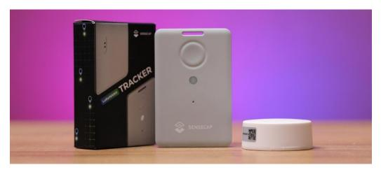
Deploy Bluetooth beacons in your target area, the tracker receives the signal sent by the beacon, and the positioning accuracy is at the meter level (2-3 meters). It can realize functions such as asset tracking, route planning, reverse car search, etc., and can be integrated into applets and APPs.
