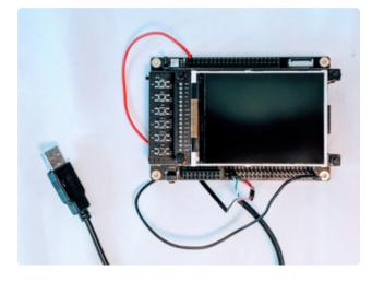
Start by connecting the USB Breakout Cable to the Kaluga board.
