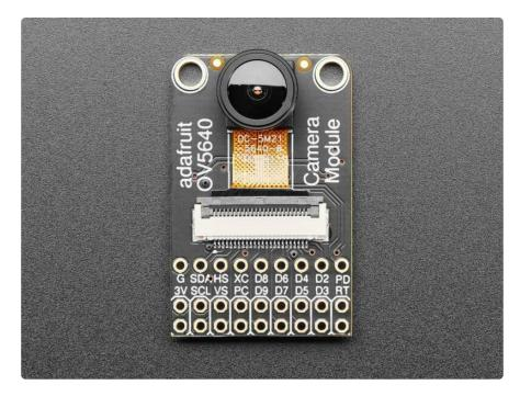
This Adafruit OV5640 Camera Breakout with 120 Degree Lens has a nice quality OV5640 camera with a 5 Megapixel sensor element, 120-degree wide angle lens, and
