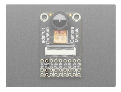
The camera module must be configured using I2C.
