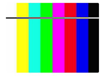
In test bar mode, the camera shows color bars in the order white - yellow - cyan green - purple - red - blue - black. A small vertical bar of inverted colors moves from top to bottom. Here's a typical test bar, captured in JPEG mode at VGA resolution.
