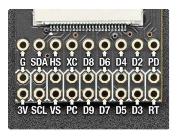
In each column, the top label (e.g., G, SDA, etc) applies to both the top and center rows of pins. The bottom label (e.g., 3V, SCL, etc) is for the bottom row of pins. As noted on the Assembly page, depending how you will install the module you will either be using the two outermost rows of pins, or the two bottom rows of pins.
