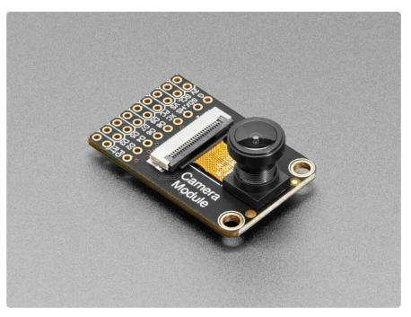
Hobby-level microcontrollers are finally getting powerful enough to start handling camera modules that historically would have required a full computer or FPGA to handle. The RP2040 and ESP32-Sx series of chips, for example, have enough pins to communicate with the 8-bit data output, DMA to quickly grab a frame, and the necessary RAM to buffer a raw snapshot. Now all that is needed is a nice camera module to make interfacing easy!
