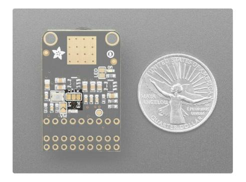
The OV5640 Camera Breakout includes an on-board 24MHz crystal oscillator. To use this as the OV5640 clock, cut the jumper from the center pad to EXT then solder between the center pad and INT. In this mode, any input on the XC pin is ignored and XC may be left unconnected.
