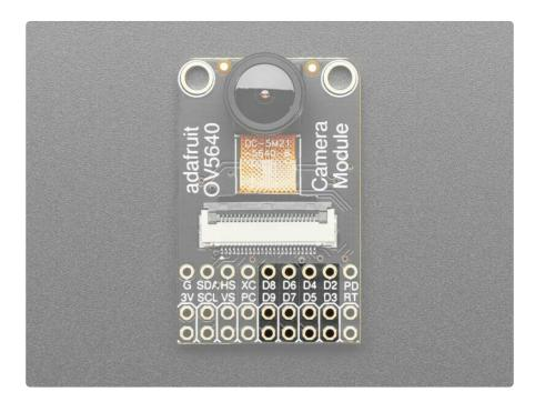
The 8 data pins (numbered from D2 to D9 because reasons) carry data out of the camera into the microcontroller.
