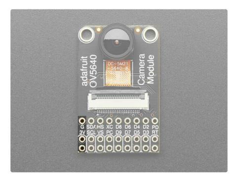
The camera module requires a well-regulated 3.3v supply in order to operate.
