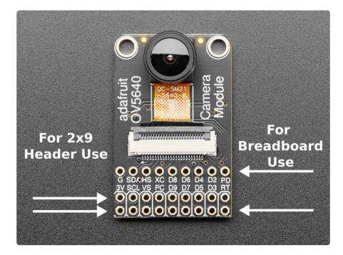
Carefully align the headers. You can use tacky clay to hold them in place. Solder just one pin in each row, then check again for alignment. If the pins are poorly aligned, reheat the solder joint while adjusting it until it is straight. Add flux if needed so that you don't end up with a cold solder joint.
