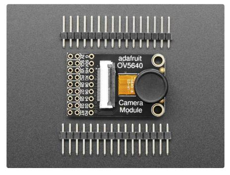
The module comes with header pins so you can solder it for use on a breadboard or on the standard 2x9 header—It's up to you.
