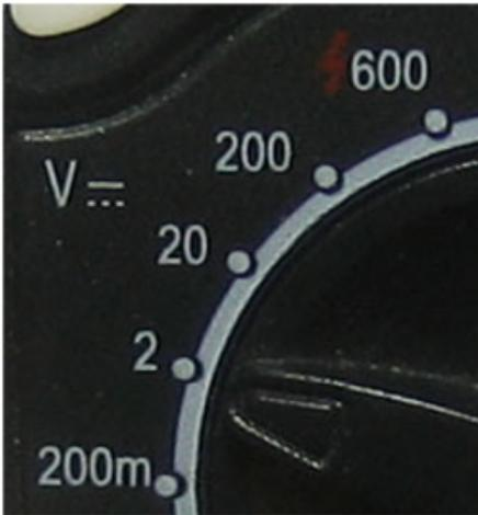
For this example, it's best to test with the output from the breakout connected to a multimeter in DC voltage mode. DC voltage mode is labeled with a V and two lines, one dashed and one solid. [For information on using a multimeter, check out this guide. \(\)](#)
