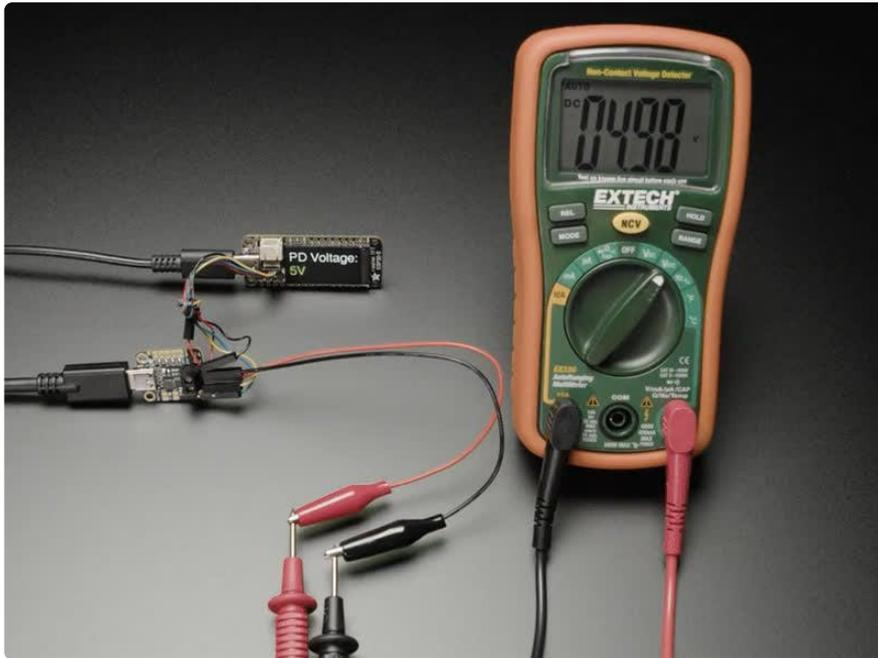
The HUSB238 USB PD sink chip is neat in that you can either use jumpers (really, resistor selection) to set the desired power delivery voltage and current or you can use I2C for dynamic querying and setting.
