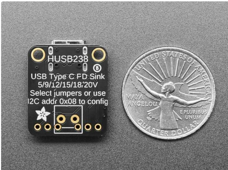
Jumper-configured usage is simple: by default its hard-wired for 5V 1A output since that's what USB C will always provide at first. Cut the 5V jumper and solder closed the 9V, 12V, 15V, 18V or 20V jumper to select the resistor that sets the voltage. You can also select the desired current from 2A to 3A, although we have found that this isn't as essential, you could always just pull as much as the adapter will provide. No microcontroller or microcomputer is required!
