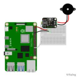
Pi 3.3V to driver VIN (red wire) Pi GND to driver GND (black wire) Pi GPIO 5 to driver SIG (white wire) Driver VO+ to piezo positive (red wire) Driver VO- to piezo negative (black wire)
