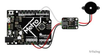
Board 5V to driver VIN (red wire) Board GND to driver GND (black wire) Board pin 5 to driver SIG (white wire) Driver VO+ to piezo positive (red wire) Driver VO- to piezo negative (black wire)
