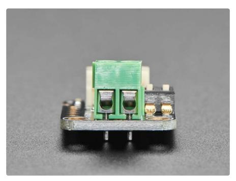
Please note: If you are powering the driver from 5VDC, don't set the gain to x3 because the 15V output is higher than the driver is specified for. (Yeah we also sorta wondered why the chip manufacturer allows it). So if you are using 3.3V power, x3 gain is OK and will give you about 10V out but if you're powering with 5V use 2x gain max to keep the max voltage at 10V.
