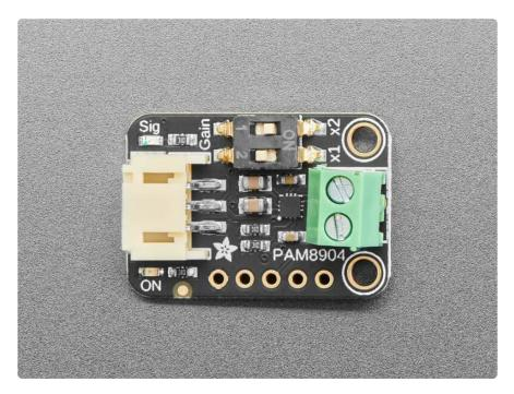
We found the nifty <u>PAM8904</u> (), which is an amplifier specifically designed for driving piezo elements - and unlike audio amplifiers, it's good for up to 300 KHz! It's a
