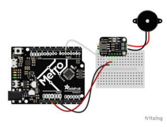
Board 5V to driver VIN (red wire) Board GND to driver GND (black wire) Board pin 5 to driver SIG (white wire) Driver VO+ to piezo positive (red wire) Driver VO- to piezo negative (black wire)
