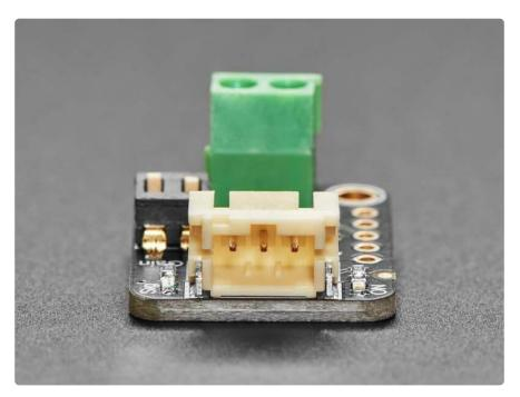
Usage is easy: power with 3 to 5VDC on the Vin and GND pins. Then provide a square wave on the signal pin, from 20Hz to 300KHz - any duty cycle is ok but 50% will probably work best. There's a dual DIP switch to set the gain: you can set it to off (zero gain), x1 gain, x2 gain and x3 gain. The output is differential, so 2x gain will give you 4xVin peak-to-peak across the piezo lines. Connect your piezo to the terminal block and you're ready to rock.
