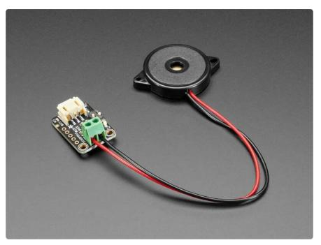
Piezos make noise when you put an AC voltage across them - and the bigger the voltage, the louder they are. With your standard 3V logic microcontroller you can make 3 volts peak to peak (Vpp) with a PWM out, or 6Vpp differential with two complementary outputs. But what if you want even louder? Or if you're using a piezo to sense distance using ultrasonic bounces?
