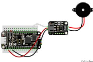
Board 3.3V to driver VIN (red wire) Board GND to driver GND (black wire) Board pin 5 to driver SIG (white wire) Driver VO+ to piezo positive (red wire) Driver VO- to piezo negative (black wire)
