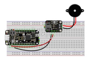
Board 3.3V to driver VIN (red wire) Board GND to driver GND (black wire) Board pin 5 to driver SIG (white wire) Driver VO+ to piezo positive (red wire) Driver VO- to piezo negative (black wire)
