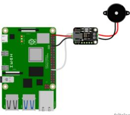
Pi 3.3V to driver VIN (red wire) Pi GND to driver GND (black wire) Pi GPIO 5 to driver SIG (white wire) Driver VO+ to piezo positive (red wire) Driver VO- to piezo negative (black wire)
