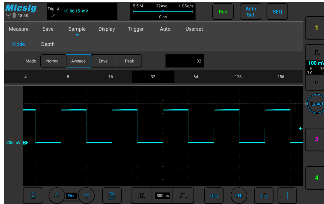
Figure 11-7 Waveform after choosing the average sampling mode, with average number 32
