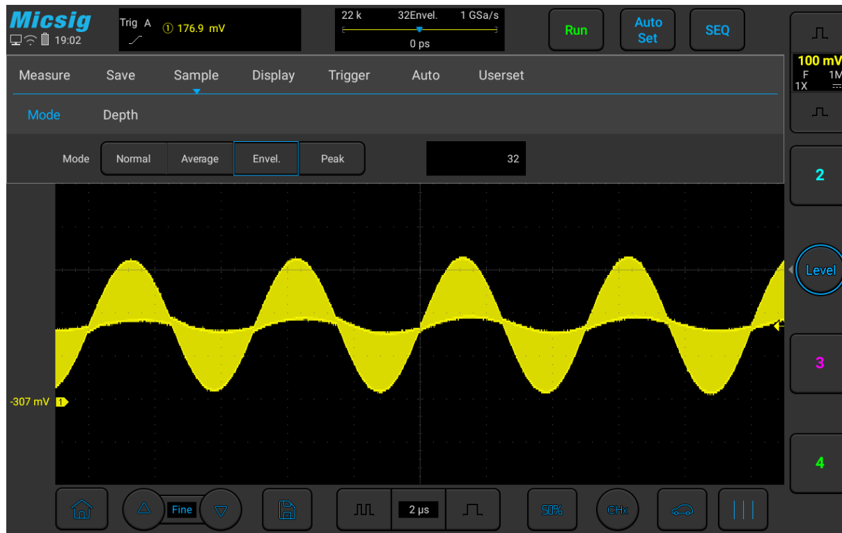
Figure 11-8 AM Signal in Envelope Sampling Mode (32)
