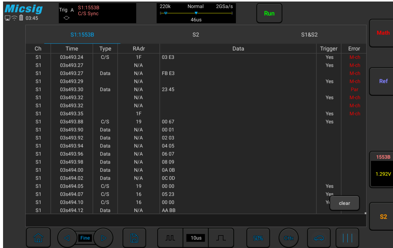
Figure 12-33 1553B Text Interface
