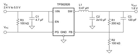
Figure 9-1. Typical Application of TPS62826x
