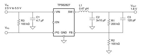
Figure 9-2. Typical Application of TPS62827
