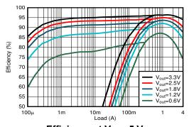
Efficiency at V<sub>IN</sub> = 5 V
