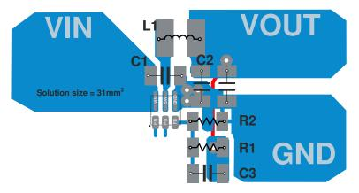
Figure 9-49. PCB Layout Recommendation
