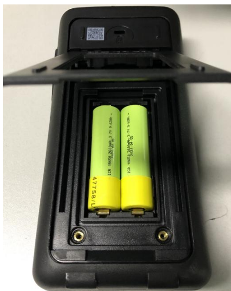
Figure 48 Installing the Battery
