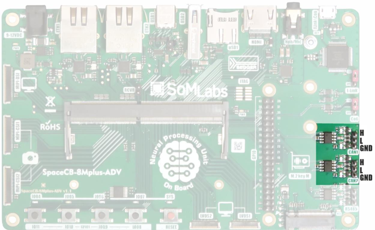
The SpaceCB-8Mplus-ADV board is equipped with Microchip CAN-FD with physical layer interfaces MCP2542FD-E/SN, connected to internal CAN1 and CAN2 channels.
