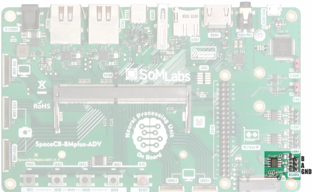
The SpaceCB-8Mplus-ADV board is equipped with low-voltage RS-485 physical layer interface MAX3485. The RS-485 is connected to default UART2 (Tx, Rx) channel and pins. Transmission control line DE is controlled by MPU GPIO.
