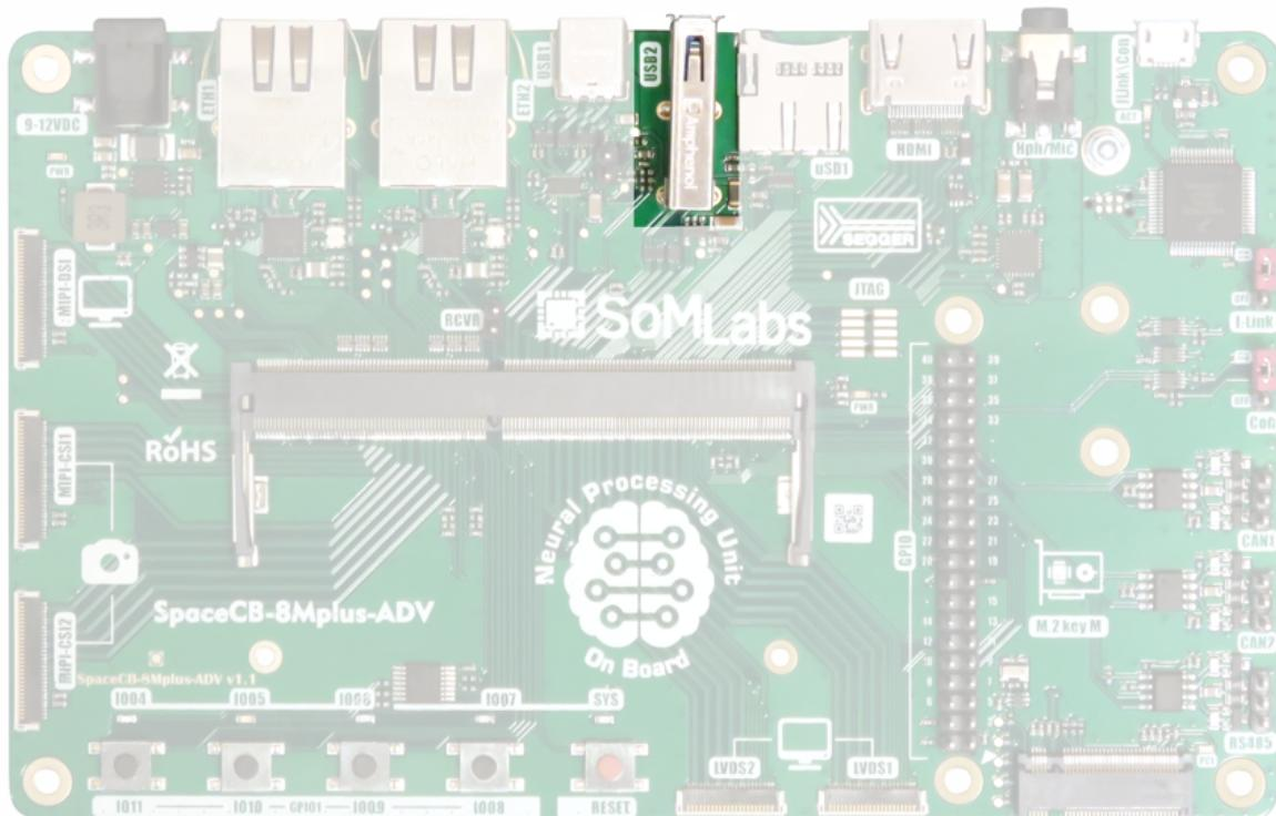
USB 3.0 interface built-in SpaceCB-8Mplus-ADV is connected to USB2 channel.
