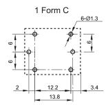
Remark: 1) In case of no tolerance shown in outline dimension: outline dimension ≤1mm, tolerance should be ±0.2mm; outline dimension >1mm and ≤5mm, tolerance should be ±0.3mm; outline dimension >5mm, tolerance should be ±0.4mm.
