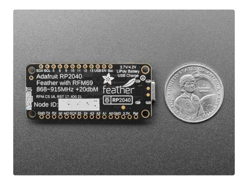
It's kinda like we took our RP2040 Feather () and RFM69 900MHz breakout board () a nd glued them together. You get all the pins for use on the Feather, the Lipoly battery support, USB C power / data, onboard NeoPixel, 8MB of FLASH for storing code and files, and then with the 8 unused pins, we wired up all the DIO pins on the RFM module. There's even room left over for a STEMMA QT connector an a uFL connector for connecting larger antennas.
