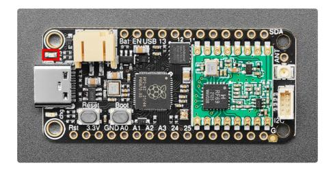
The red LED is above the USB-C connector on the left side of the board.
