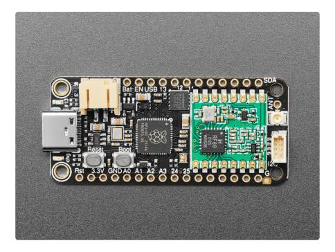
This is the Adafruit Feather RP2040 RFM69 Packet Radio (868 or 915 MHz). We call these RadioFruits, our take on an microcontroller with packet radio transceiver with built-in USB and battery charging. It's an Adafruit Feather RP2040 with a RFM69HCW 900MHz radio module cooked in! Great for making wireless networks that are more flexible than Bluetooth LE and without the high power requirements of WiFi.
