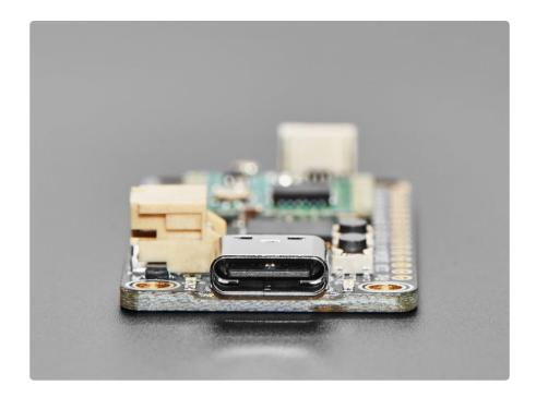
At the Feather's heart is an RP2040 chip, clocked at 133 MHz and at 3.3V logic, the same one used in the Raspberry Pi Pico (). This chip has a whopping 8MB of onboard QSPI FLASH and 264K of RAM! This makes it great for making wireless sensor nodes that can send to each other without a lot of software configuration.
