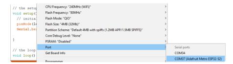
You can now select the new serial port name which will be different than the bootloader serial port. Arduino IDE will try to use auto-reset to automatically put the board into bootloader mode when you ask it to upload new code
