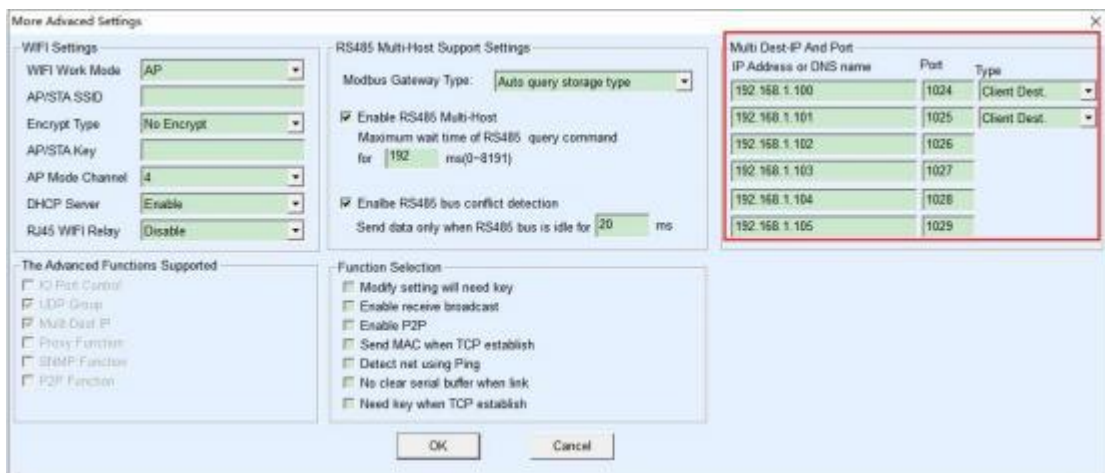
Figure 15 The remaining 2~7 IPs and ports
