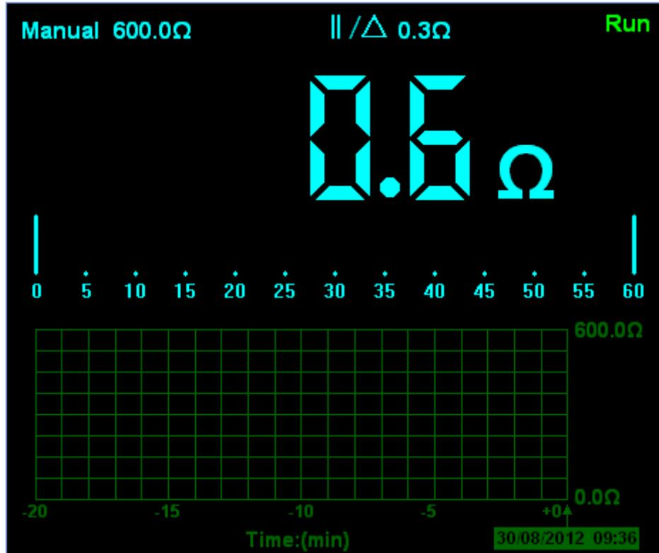
Figure 2-21 Relative Measurement
