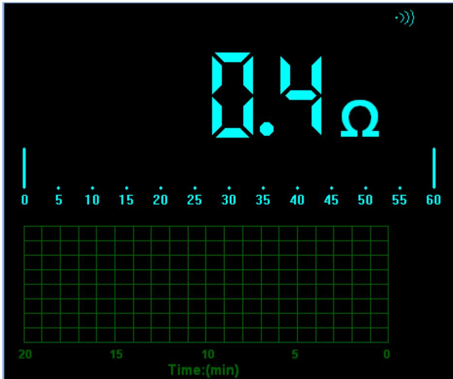
Figure 2-18 On-Off Measurement
