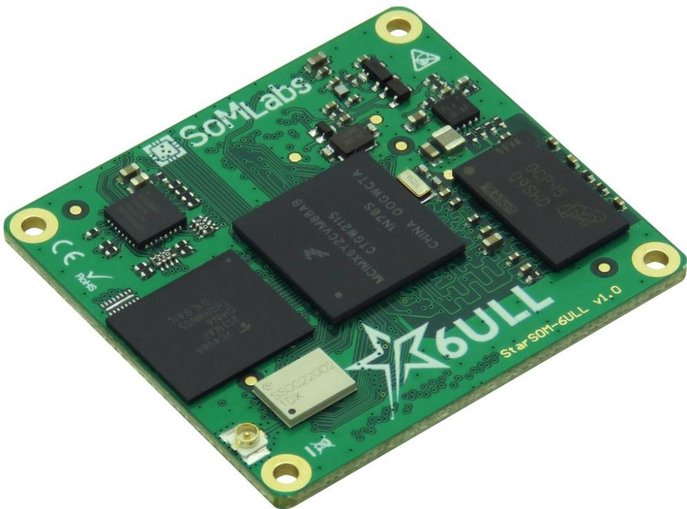
The StarSOM-6ULL family is a small size and low profile SoM based on the NXP i.MX6 ULL application processor, which features an advanced implementation of a single ARM Cortex-A7 core (at speeds up to 900MHz).
