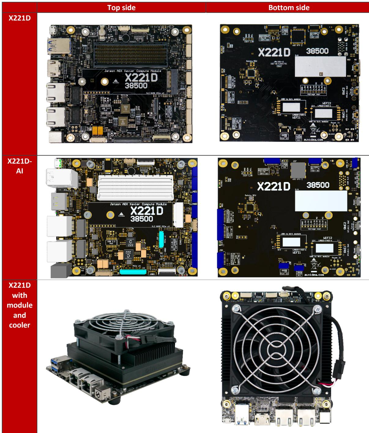
The heatsink is designed for the AGX Xavier & AGX Xavier Industrial & AGX Orin. It is designed to mount a standard 80x80mm fan. A production version is available. The Heatsink is not included with the base board. Sets may be available.
