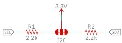
Cut traces to disconnect I2C pullup resistors
