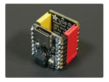
Connect the QT Py RP2040 with plug headers into the 5x5 NeoPixel Grid BFF with socket headers. They should be plugged in with the backs of the boards facing each other.
