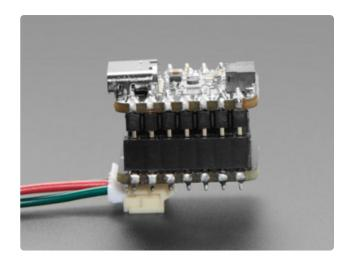
Connect the QT Py RP2040 with plug headers into the NeoPixel Driver BFF with socket headers. They should be plugged in with the backs of the boards facing each other.
