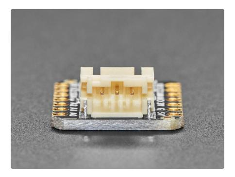
Note that we connect the USB 5V power directly out to the NeoPixel power pin on the JST PH connector and PH connectors are only rated for about 2 Amps, so it's not for powering directly more than maybe 30-60 NeoPixels (less if they're on full white brightness).
