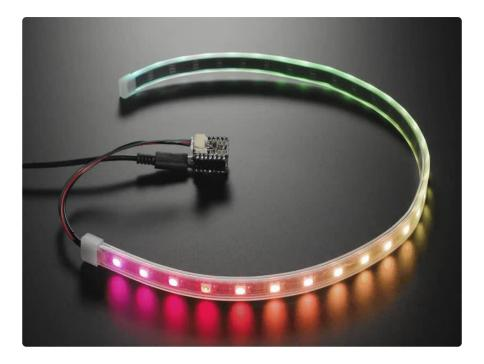
Adafruit's QT Py boards are a great way to make very small microcontroller projects that pack a ton of power - and now there is a way for you to quickly add a <u>strand of NeoPixels</u> () with a 5V level shifter and a detachable JST PH connector. It's an excellent way to make tiny wearable, cosplay or IoT projects with dazzling LEDs.
