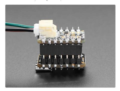
This PCB is designed to fit onto the back of any QT Py or Xiao board, it can be soldered into place or use pin and socket headers to make it removable. Onboard is a 74AHCT125 single-gate level shifter that will take pin A3's output, and shift it up to 5V using the USB power as a reference. The USB power, ground and shifted data is then piped out to a JST PH 2mm 3-pin connector.
