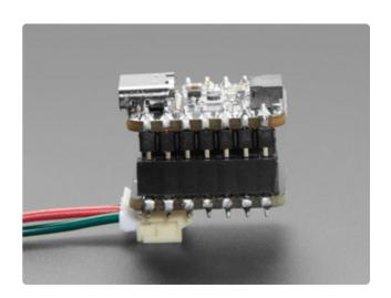
Connect the QT Py RP2040 with plug headers into the NeoPixel Driver BFF with socket headers. They should be plugged in with the backs of the boards facing each other.
