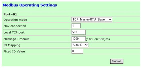
**Max connection:** The maximum number of connections allowed by Modbus TCP master station is 32. Users can adjust this parameter according to the actual application. When users do not need 32 connections, they can be reduced to improve performance. The effective range of the maximum number of connections is 1~32. You need to change this value when multiple TCP master stations or multiple RTU/ASCII slave stations.
