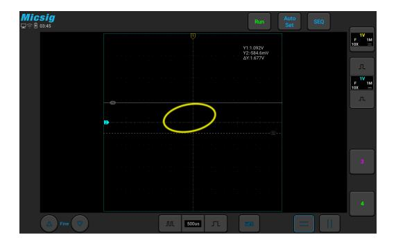
Figure 3-10 Phase Difference Measurement and Using the Cursor
