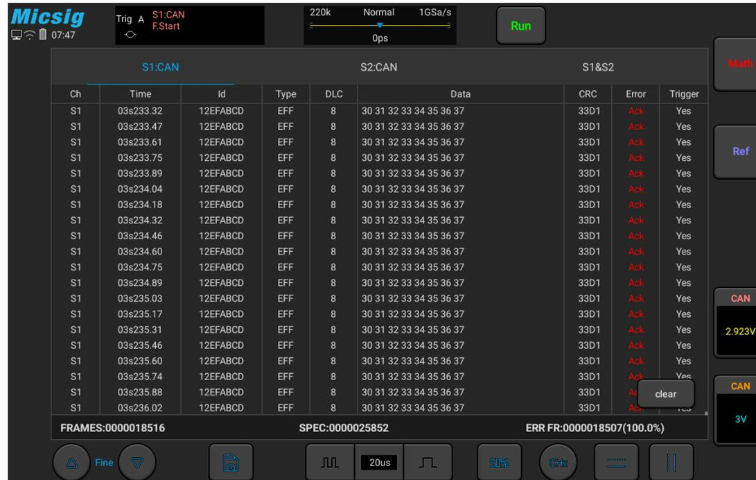
Figure 11-17 CAN Text Interface
