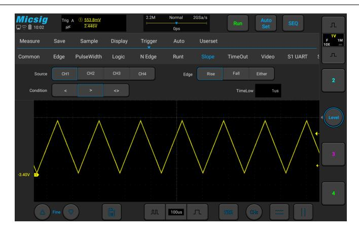
Figure 5-27 Slope Trigger Setting Menu
