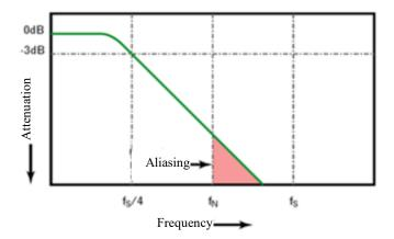
Figure 10-3 Sampling Rate and Oscilloscope Bandwidth
