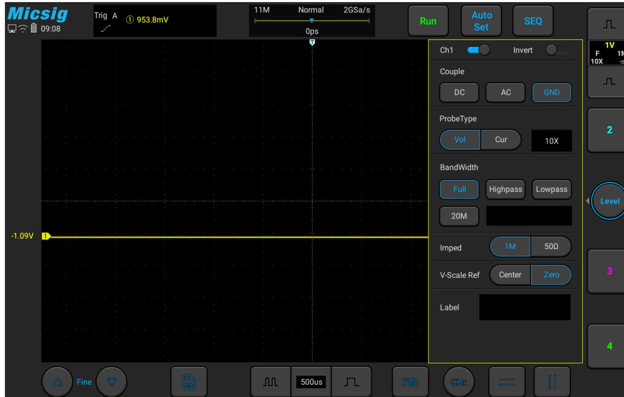
Figure 4-9 GND Coupling
