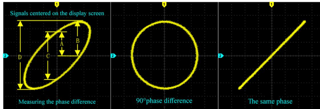
Figure 3-9 XY Time Base Mode Signal, Center on the Display Screen
