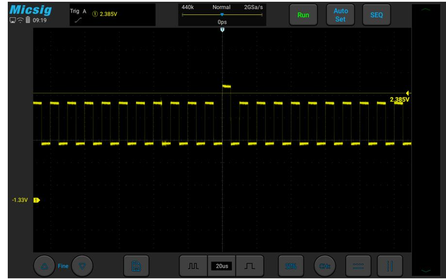
Figure 5-4 Abnormal Signal Captured by Setting Trigger Level
