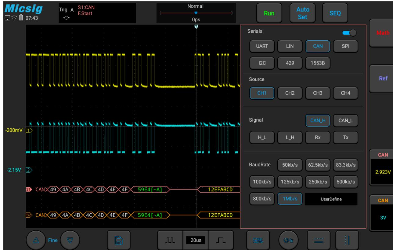
Figure 11-14 CAN Bus Configuration Menu
