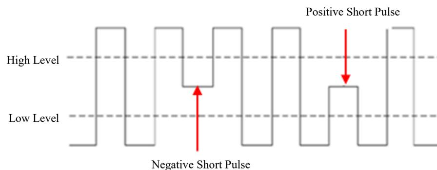
Figure 5-24 Runt Trigger
