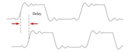
Figure 6-5 Delay Measurement Schematics
