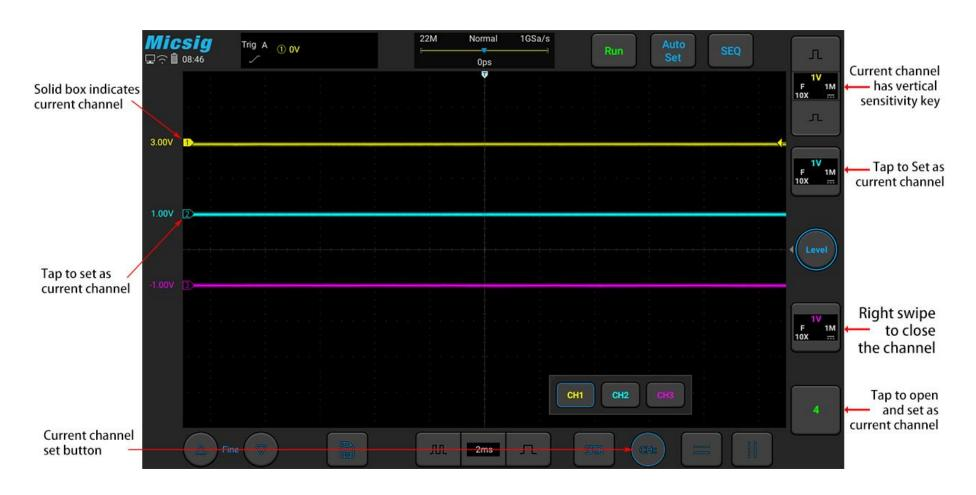
Figure 4-4 Channel Open, Close and Switching
