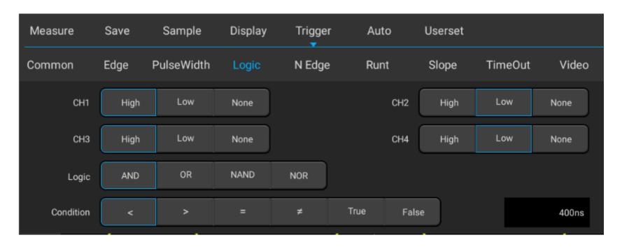
Figure 5-21 Logic Trigger Setting Menu
