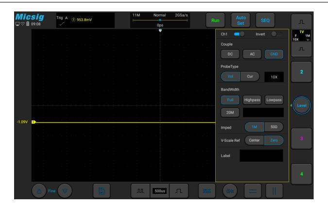
Figure 4-9 GND Coupling
