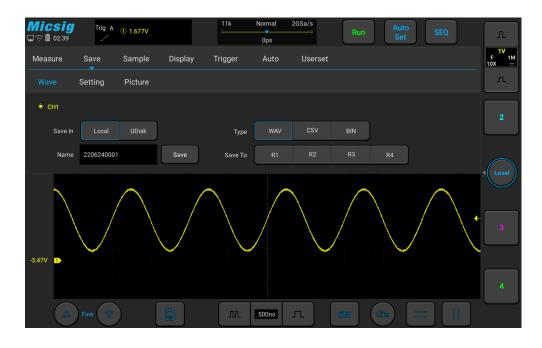
Figure 7-5 Save CH1 Reference Waveform Interface
