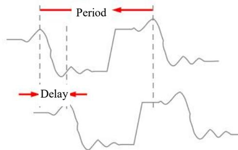
Figure 6-6 Phase Measurement Schematics
