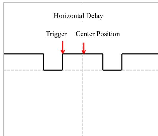
Figure 5-7 Horizontal Delay
