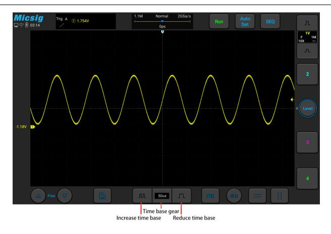
Figure 3-3 Adjust the Horizontal Time Base
