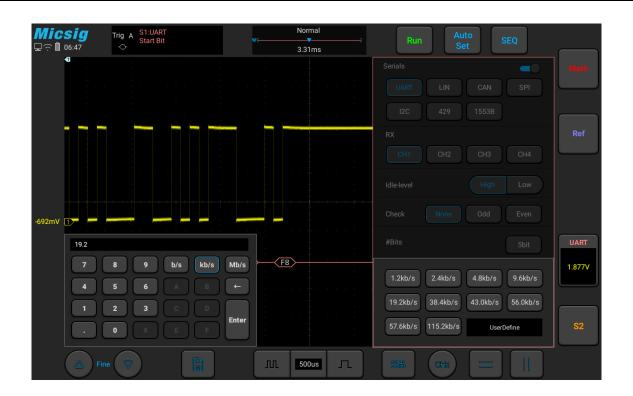
Figure 11-5 Baud Rate Default Setting
