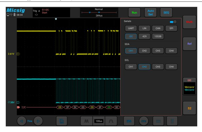
Figure 11-22 I2C Bus Configuration Menu
