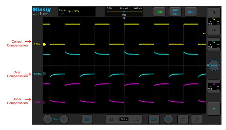
Figure 2-14 Probe Compensation
