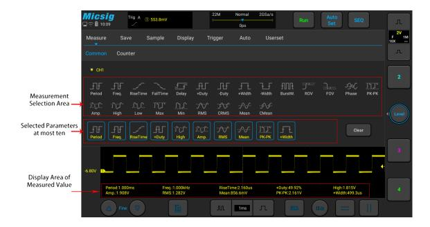
Figure 6-1 Automatic Measurement Menu
