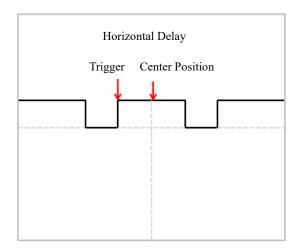
Figure 5-7 Horizontal Delay
