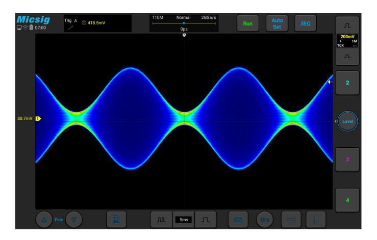
Figure 9-5 Color Temperature Open Mode
