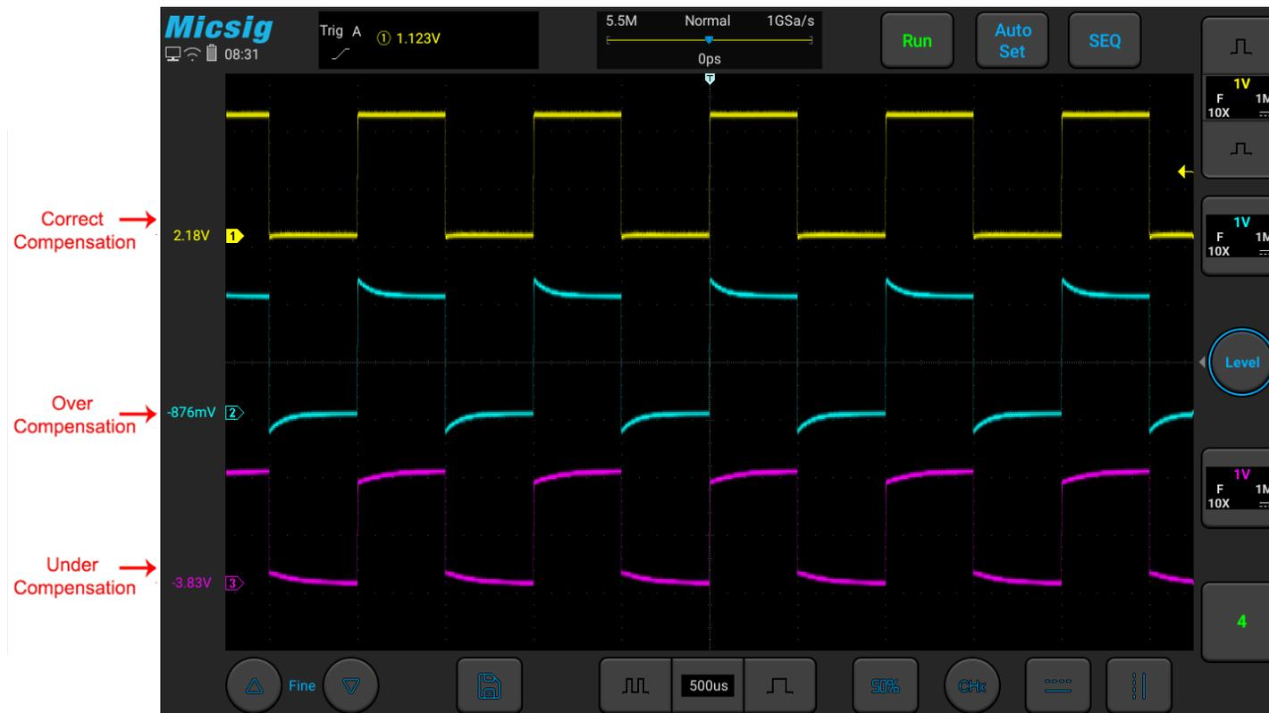
Figure 2-14 Probe Compensation
