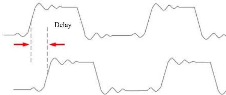
Figure 6-5 Delay Measurement Schematics
