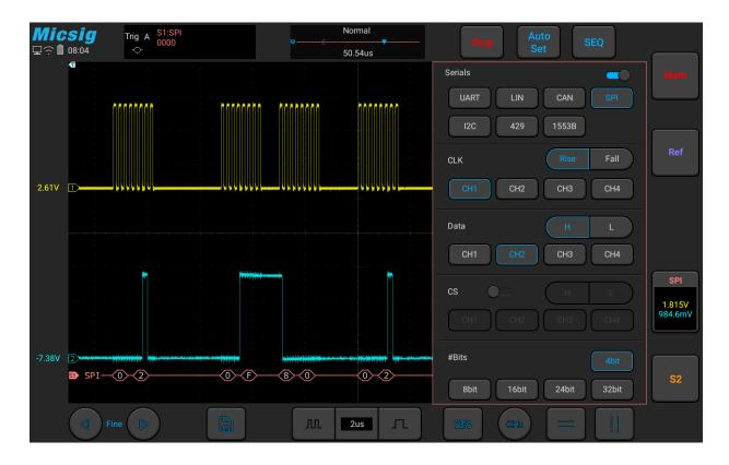
Figure 11-18 SPI Bus Configuration Menu
