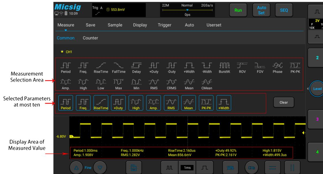
Figure 6-1 Automatic Measurement Menu
