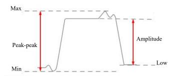
Figure 6-7 Voltage Measurement
