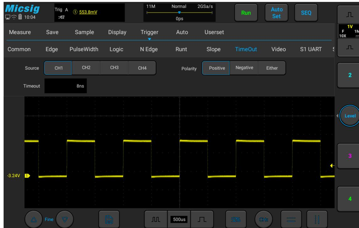
Figure 5-29 Time-out Trigger
