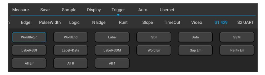
Figure 11-27 ARINC429 Trigger Mode Configuration Menu
