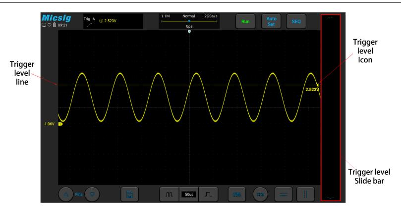
Figure 5-8 Trigger Level
