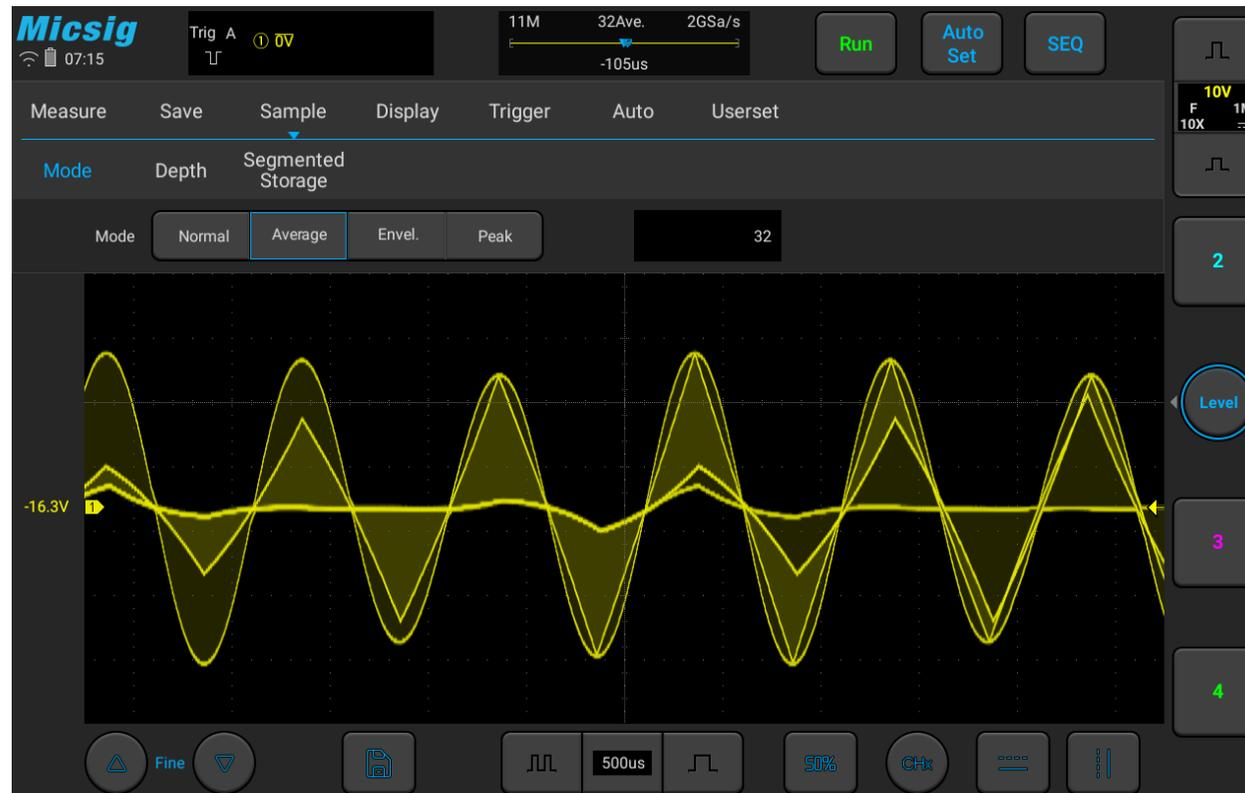
Figure 10-8 AM Signal in Envelope Sampling Mode (32)
