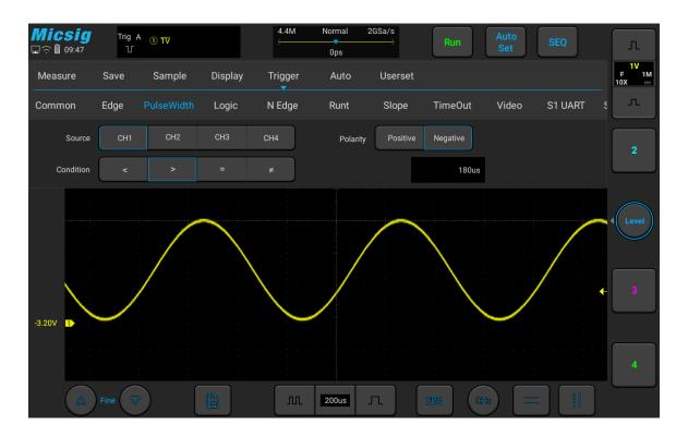
Figure 5-15 Negative Polarity Pulse Level Flip
