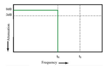
Figure 10-2 Theoretical Brick-Wall Frequency Response
