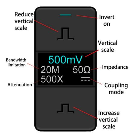
Figure 4-3 Channel Display Interface
