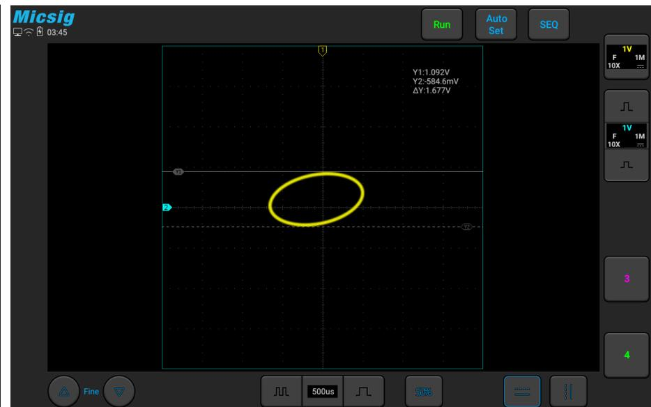
Figure 6-13 In XY Mode, Cursor Measurement
