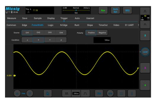
Figure 5-14 Pulse Width Trigger Setting Menu
