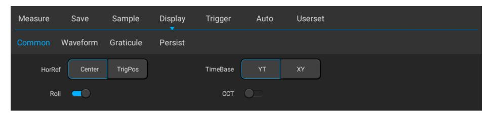
Figure 9-1 Display Settings and Function Buttons
