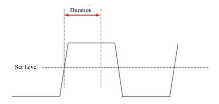
Figure 5-28 Timeout Trigger Schematics
