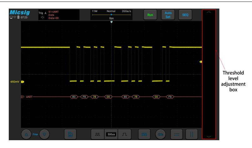
Figure 11-7 UART Decode Level Adjustment
