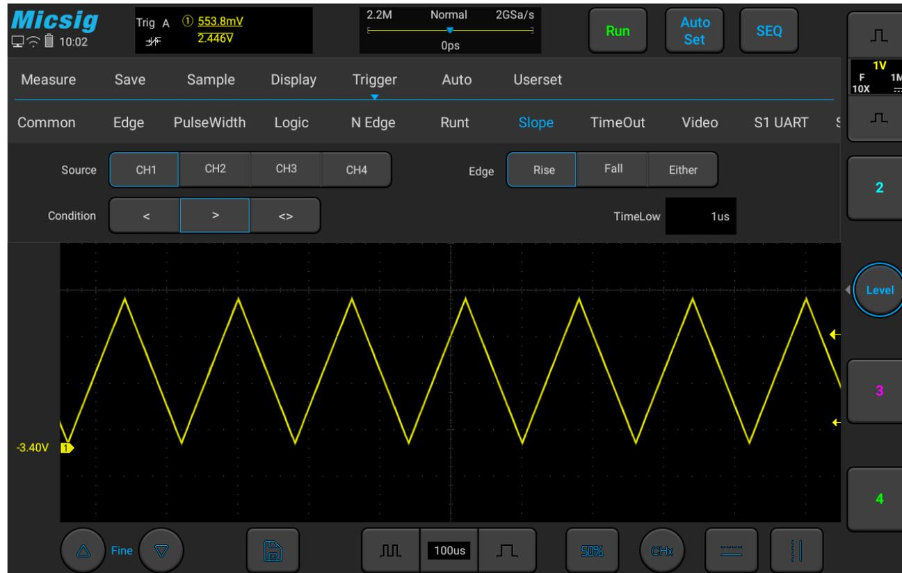
Figure 5-27 Slope Trigger Setting Menu
