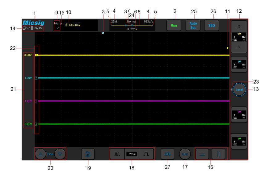
Figure 2-6 Oscilloscope Interface Display
