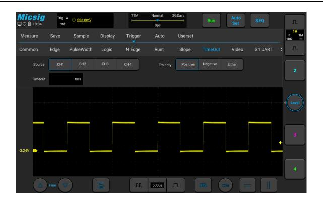
Figure 5-29 Time-out Trigger
