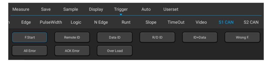
Figure 11-15 CAN Trigger Mode Configuration Menu
