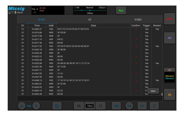
Figure 11-25 I2C Text Interface
