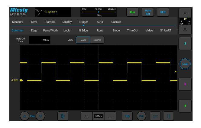
Figure 5-5 Oscilloscope Trigger Mode Setting
