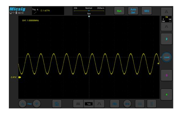
Figure 6-9 Frequency Meter Measurement
