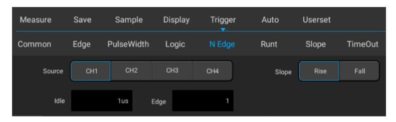
Figure 5-12 Edge Trigger Setting Menu
