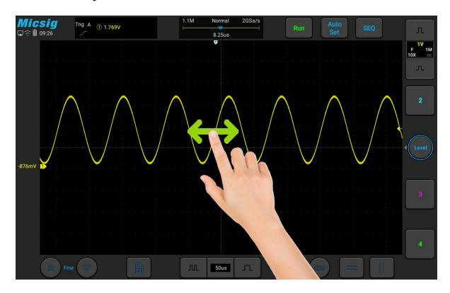
Figure 3-2 Move the Waveform Horizontally on the Screen
