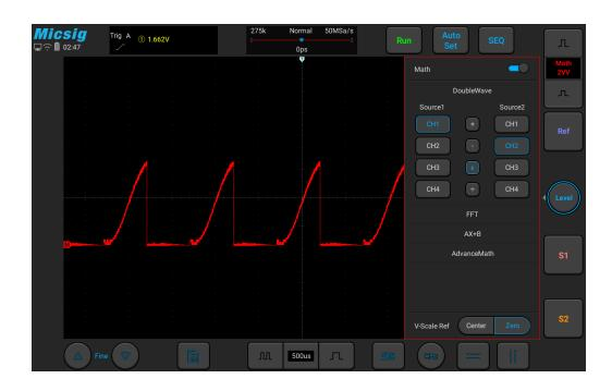
Figure 8-1 MATH Channel Waveform
