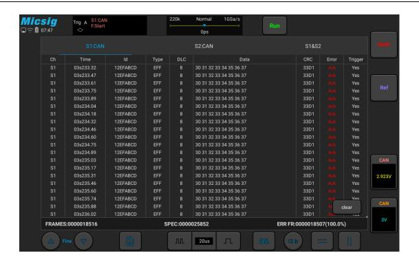
Figure 11-17 CAN Text Interface
