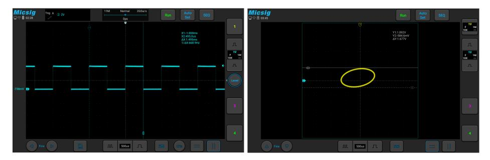
Figure 6-12 Cursor Measurement Pulse Width
