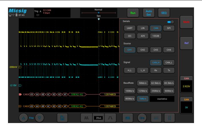
Figure 11-14 CAN Bus Configuration Menu
