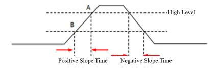
Figure 5-26 Positive/Negative Slope Time
