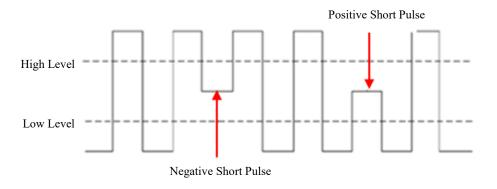
Figure 5-24 Runt Trigger
