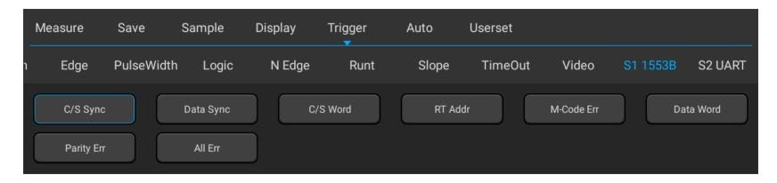
Figure 11-31 1553B Trigger Mode Configuration Menu
