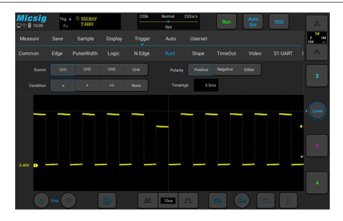
Figure 5-25 Runt Trigger Setting Menu
