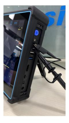
Figure 2-13 Probe Connection
