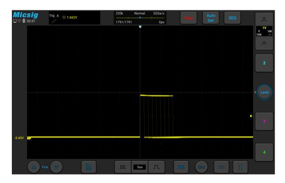
Figure 10-11 Segmented memory waveform acquisition
