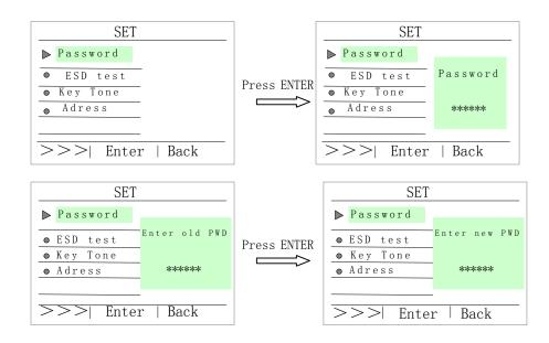
△ Note: after change password, the temperature cannot be modify, enter into parameter setting interface with new right password.
