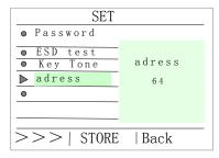
2.After setting , press "STORE" save, and press "Back" key return parameter setting interface, and press "Back" key return main menu.
