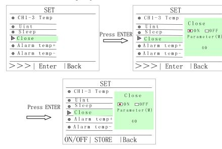
2. After setting close time ,press "STORE" key affirm, press "Back" key return parameter setting interface, press "Back" again, return setting interface.
