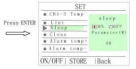
⚠ Note: The range of sleep time is between 5S and 99 minute, Press any key button can awake sleep. If sleep 60 minute nonactivated, it will auto power-off.
