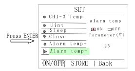
2. After setting alarm temperature-, press "store" affirm, press "Back" return parameter setting interface, press "Back" again, return menu interface.
