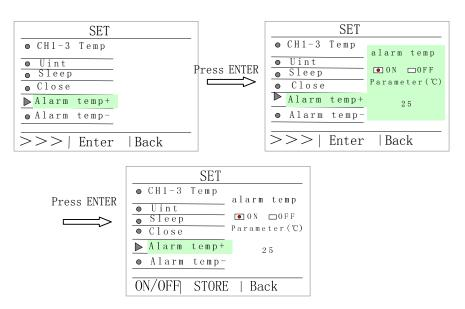
2. after setting alarm temperature+, press "store" affirm, press "Back" return parameter setting interface, press "Back" again, return menu interface.
