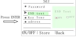
△ Note: when select ON, the ground hole must be connect with ESD ground, otherwise, alarm hint (ESD in main interface show as red)
