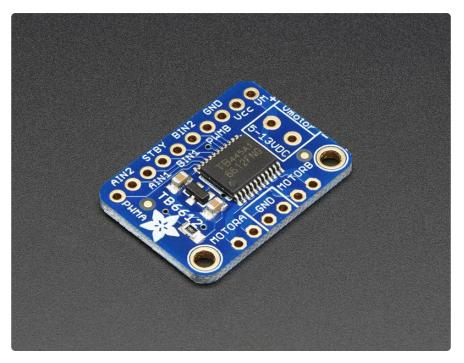
Fire four solenoids, spin two DC motors or step one bi-polar or uni-polar stepper with 1.2A per channel using the TB6612. These are perhaps better known as "the drivers in our assembled Adafruit Motorshield (http://adafru.it/1438) or Motor HAT ()" We really like these dual H-bridges, so if you want to control motors without a shield or HAT these are easy to include on any solderless breadboard or perma-proto.
