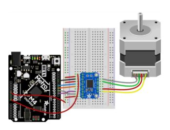
Board VM to Metro VIN Board VCC to breadboard power rail Board GND to Metro GND Board PWMB to breadboard power rail Board BIN2 to Metro D12 Board BIN1 to Metro D11 Board AIN1 to Metro D9 Board AIN2 to Metro D10 Board PWMA to breadboard power rail Breadboard power rail to Metro 5V Board MOTORA (two pins) to stepper coil (red and yellow stepper wires) Board MOTORB (two pins) to stepper coil (green and grey stepper wires) 9V power supply to barrel jack on Metro
