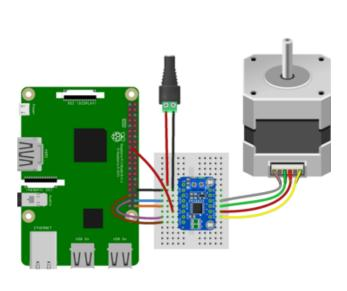
Board VM to positive terminal on barrel jack Board GND to negative terminal on barrel jack Barrel jack to 9V power supply Board GND to Pi GND Board SLP to Pi 3.3V Board AIN1 to Pi D19 Board AIN2 to Pi D26 Board BIN2 to Pi D21 Board BIN2 to Pi D21 Board AOUT (1 and 2) to stepper coil (red and yellow stepper wires) Board BOUT (1 and 2) to stepper coil (green and grey stepper wires)
