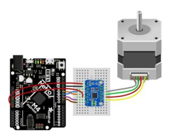
Board VM to Metro VIN Board GND to Metro GND Board SLP to Metro 5V Board AIN1 to Metro D9 Board AIN2 to Metro D10 Board BIN1 to Metro D11 Board BIN2 to Metro D12 Board AOUT (1 and 2) to stepper coil (red and yellow stepper wires) Board BOUT (1 and 2) to stepper coil (green and grey stepper wires) 9V power supply to barrel jack on Metro
