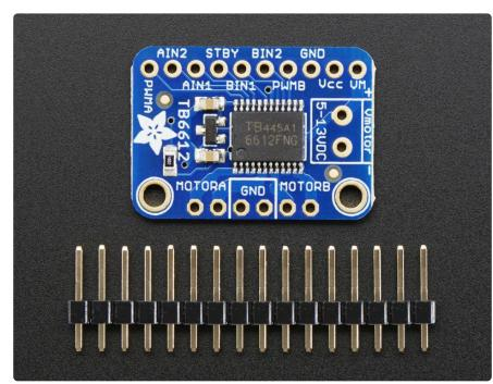
This motor driver is a fairly simple breakout of the TB6612 motor chip, so do check out the datasheet for the TB6612 for any details you need about pin voltage limits, capacitance, etc! ()
