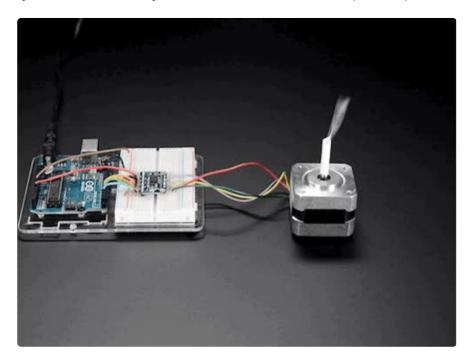
We solder on TB6612 onto a breakout board for you here, with a polarity protection FET on the motor voltage input and a pullup on the "standby" enable pin. Each
