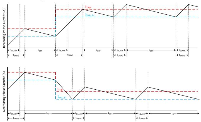
Figure 7-5. Smart tune Ripple Control Decay Mode
