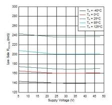
Figure 6-6. Low-Side  $R_{DS(ON)}$  over Supply Voltage
