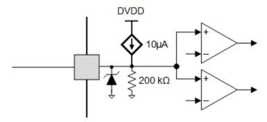
Figure 7-8. Tri-Level Input Pin Diagram
