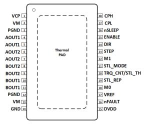
Figure 5-1. PWP PowerPAD™ Package 28-Pin HTSSOP Top View
