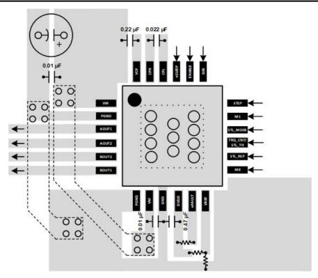
Figure 10-2. QFN Layout Example
