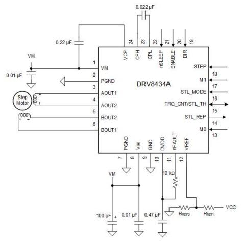
Figure 8-2. Typical Application Schematic (VQFN package)
