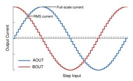
Figure 7-1. Full-Scale and RMS Current
