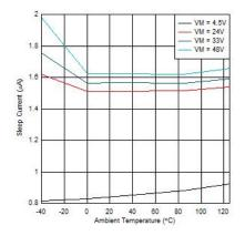
Figure 6-3. Sleep Current over Temperature
