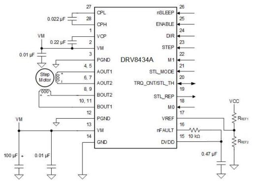
Figure 8-1. Typical Application Schematic (HTSSOP package)
