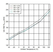
Figure 6-7. Low-Side R<sub>DS(ON)</sub> over Temperature
