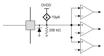
Figure 7-9. Quad-Level Input Pin Diagram
