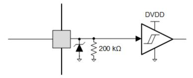
Figure 7-10. Logic-Level Input Pin Diagram
