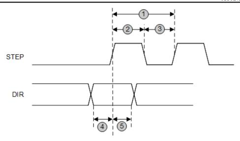
Figure 6-1. STEP and DIR Timing Diagram
