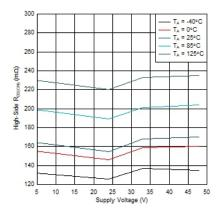
Figure 6-8. High-Side  $R_{DS(ON)}$  over Supply Voltage
