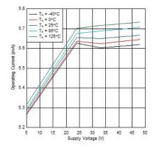
Figure 6-4. Operating Current over Supply Voltage
