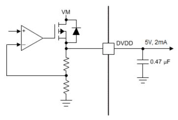
Figure 7-7. Linear Voltage Regulator Block Diagram
