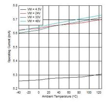
Figure 6-5. Operating Current over Temperature
