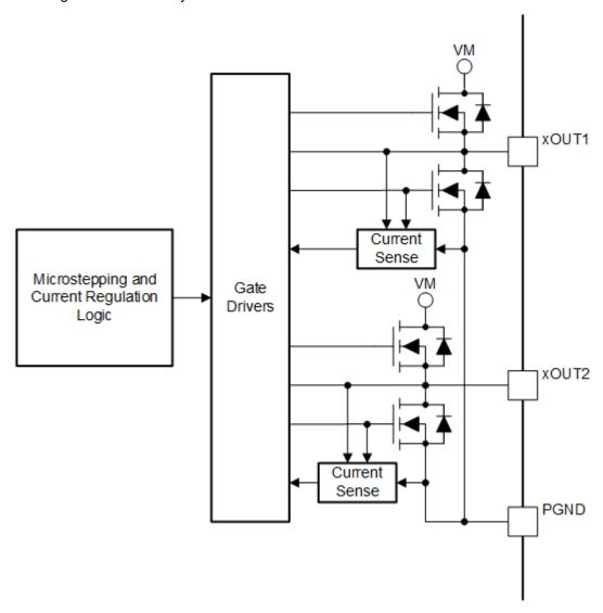
Figure 7-2. PWM Motor Driver Block Diagram
