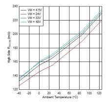
Figure 6-9. High-Side R<sub>DS(ON)</sub> over Temperature
