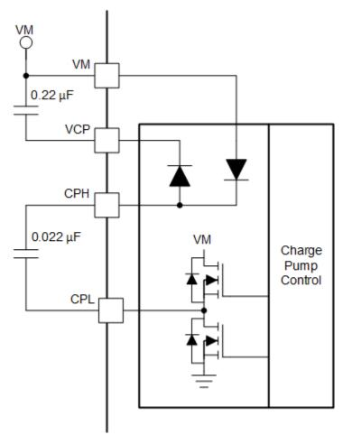
Figure 7-6. Charge Pump Block Diagram
