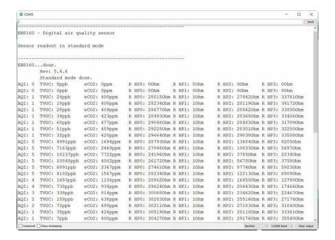
Upload the sketch to your board and open up the Serial Monitor (Tools -> Serial Monitor) at 115200 baud. You should see that the sketch has found your connected I2C ENS160 gas sensor. Then, sensor readings for AQI, TVOC, eCO2 and the raw resistance values of the four hot plates in the sensor are printed to the Serial Monitor every second.
