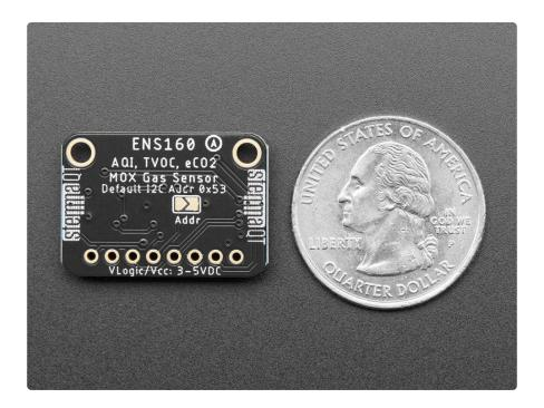
The ENS160 has a 'standard' hot-plate MOX sensor, as well as a small microcontroller that controls power to the plate, reads the analog voltage, and provides an I2C interface to read from. ScioSense provides an Arduino library with examples of reading the four raw resistance values and also the TVOC and eCO2 (https://adafru.it/PaX) and a Python/CircuitPython library (https://adafru.it/11dZ) that can be used with Linux computers like the Raspberry Pi or our CircuitPython boards.
