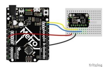
Board 5V to sensor VIN (red wire)
