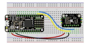
Board 3V to sensor VIN (red wire)
