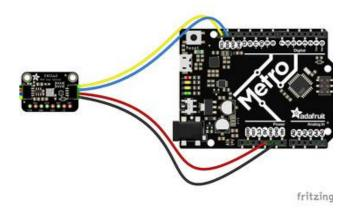
Board 5V to sensor VIN (red wire)
