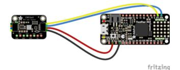
Board 3V to sensor VIN (red wire)
