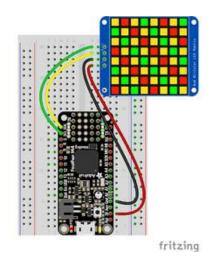
Microcontroller 3V to LED Matrix VIN Microcontroller GND to LED Matrix GND Microcontroller SCL to LED Matrix SCL Microcontroller SDA to LED Matrix SDA
