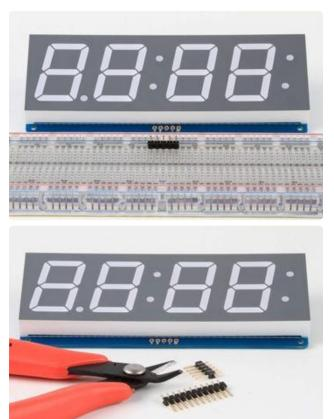
Cut the header strip to length if necessary and insert LONG pins down into the breadboard.
