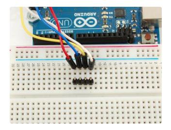
Now you're ready to wire it up to a microcontroller. We'll assume you want to use a 4pin header. You can also of course solder wires directly. Place a 4-pin piece of header with the LONG pins down into the breadboard.
