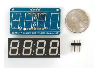
When you buy a pack from Adafruit, it comes with the fully tested and assembled backpack as well as a 7-segment display in one of the colors we provide (say, red, yellow, blue or green). You'll need to solder the matrix onto the backpack but it's an easy task.
