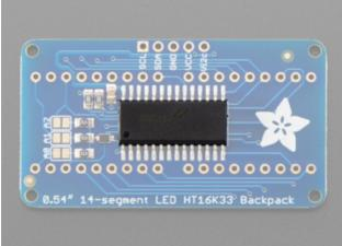
The chip located in the center of the back of the backpack is the HT16K33 matrix driver, which drives the 14-segment LED displays.
