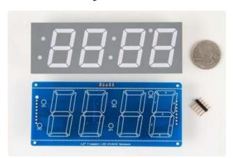
When you buy a pack from Adafruit, it comes with the fully tested and assembled backpack as well as a 7-segment display in one of the colors we provide (say, red, yellow, blue or green). You'll need to solder the matrix onto the backpack but its an easy task.
