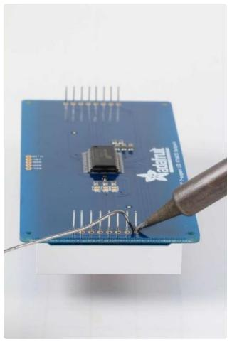
Then solder each pin. There are 8 on each end for a total of 16.
