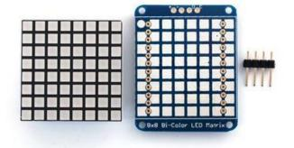
When you buy a pack from Adafruit, it comes with the fully tested and assembled backpack as well as a 8x8 matrix. You'll need to solder the matrix onto the backpack but its an easy task.
