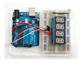
Connect CLK to the I2C clock - on Arduino UNO thats Analog #5 (or SCL), on the Leonardo it's Digital #3, on the Mega it's digital #21
