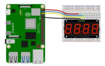
Raspberry Pi 3.3V to 7-Segment Display VIN (red wire)
