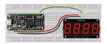
Microcontroller 3V to 7-Segment Display VIN (red wire)
