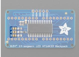
On the back of the board are three address jumpers, labeled AO, A1, and A2. These jumpers allow you to chain up to 8 of these boards on the same pair of I2C clock and data pins. To do so, you solder the jumpers "closed" in various combinations by connecting the two pads.
