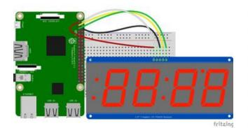
Raspberry Pi 3.3V to 7-Segment Display IO
