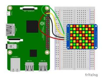
Raspberry Pi 3.3V to LED Matrix VIN Raspberry Pi GND to LED Matrix GND Raspberry Pi SCL to LED Matrix SCL Raspberry Pi SDA to LED Matrix SDA
