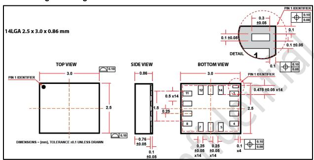
Figure 22. 14 Pin LGA 2.5 x 3.0 x 0.86 mm Package
