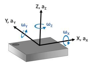
Figure 7. Chip Orientation Coordinate System
