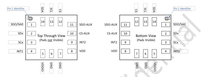
Figure 4. Pins Face Down (Top View)
