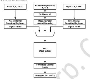
Figure 9. FIFO Data Flow
