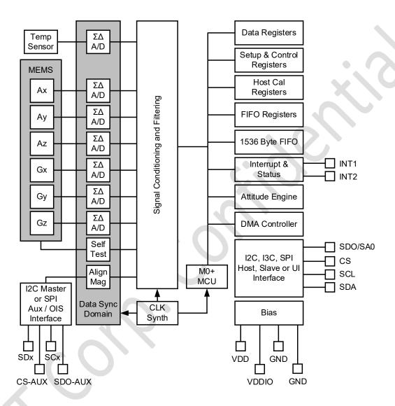
Figure 2. Internal Block Diagram
