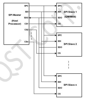
Figure 13. Typical SPI 4-Wire Multi-Slave
