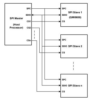
Figure 14. Typical SPI 3-Wire Multi-Slave
