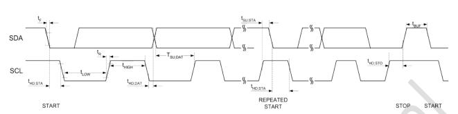
Figure 20. I<sup>2</sup>C Standard Mode Interface Timing
