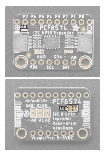
On the left side of the front of the board is the on LED which lights up when the board has power. It is labeled above the LED as on.
