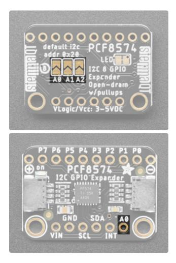
On the back of the board are three address jumpers, labeled A0, A1, and A2. These jumpers allow you to chain up to 8 of these boards on the same pair of I2C clock and data pins. To do so, you solder the jumpers "closed" by connecting the two pads.
