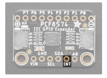
The INT pin is the IRQ output, which will automatically alert you when input pins change value.
