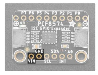
VIN - This is the power pin. To power the board, give it the same power as the logic level of your microcontroller - i.e. for a 5V micro like Arduino, use 5V, or for a 3V micro like a Feather, use 3V. GND - This is common ground for power and logic.
