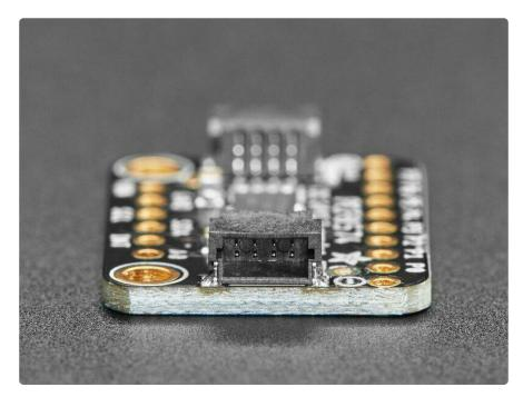
To get you going fast, we spun up a custom-made PCB in the <u>STEMMA QT form</u> factor (https://adafru.it/LBQ), making it easy to interface with. The <u>STEMMA QT</u> connectors (https://adafru.it/JqB) on either side are compatible with the SparkFun
