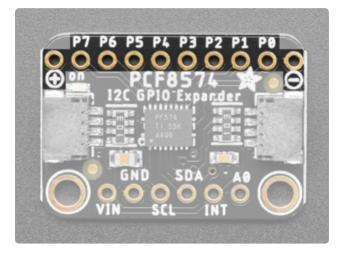
Along the top are the 8 I/O pins for expanding your project. They are labeled above the pads, left-to-right as P7 through P0.
