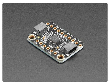
GPIO expanders work like this: you have a board with some number of GPIO but not enough for your project - maybe you need more buttons or LEDs. You could upgrade to a board with massive number of GPIO like the Grand Central (https://adafru.it/QtD), or you could pop on one of these boards.
