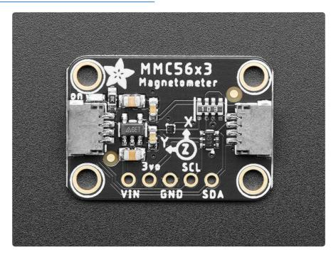
We based this breakout on the MMC5603, a great general purpose magnetometer with a very wide range and both I2C and SPI interfaces. This compact sensor is very easy to use. Simply download our library and connect the SCL pin to your I2C clock pin, and SDA pin to your I2C data pin and upload our test program to read out magnetic field data. If you'd like, you can also use SPI to receive data (we just happen to prefer I2C here).
