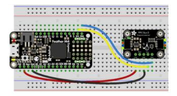
Board 3V to sensor VIN (red wire) Board GND to sensor GND (black wire) Board SCL to sensor SCL (yellow wire) Board SDA to sensor SDA (blue wire)
