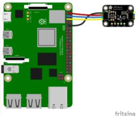
Pi 3V to sensor VIN (red wire) Pi GND to sensor GND (black wire) Pi SCL to sensor SCL (yellow wire) Pi SDA to sensor SDA (blue wire)
