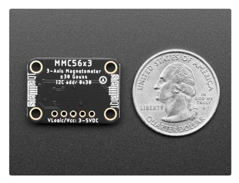
This sensor can sense ranges from ±30 Gauss (±3000uT or ±3mT) with no rangesetting required and full 20 bit output, up to 1000 Hz rate reading. The range makes it good for reading Earth's magnetic field (which maxes at about 0.6 Gauss) or some basic magnets. It isn't good for very strong rare earth magnets, for that check out the TLV293 (https://adafru.it/IES).
