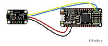
Board 3V to sensor VIN (red wire) Board GND to sensor GND (black wire) Board SCL to sensor SCL (yellow wire) Board SDA to sensor SDA (blue wire)
