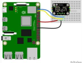
Pi 3V to sensor VIN (red wire) Pi GND to sensor GND (black wire) Pi SCL to sensor SCL (yellow wire) Pi SDA to sensor SDA (blue wire)
