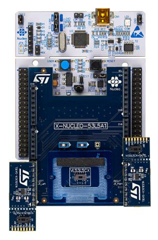
Figure 2. Connections of VL53L5CX breakout boards
