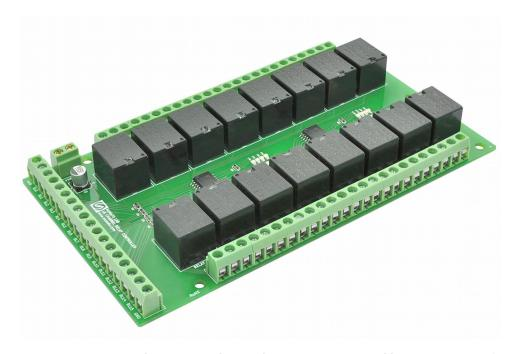
16 Channel Relay Controller Board
