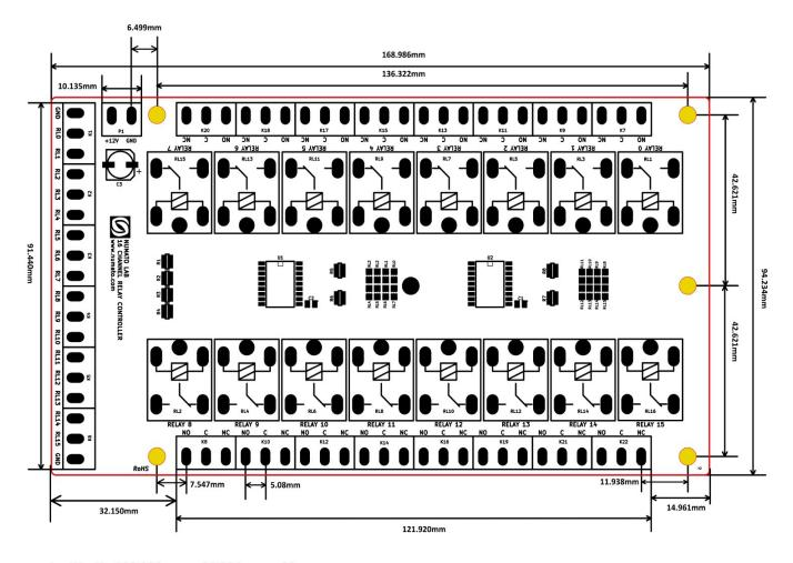
L x W x H : 168.986 mm x 94.234 mm x 20 mm Mechanical Hole Diameter : 4.0 mm
