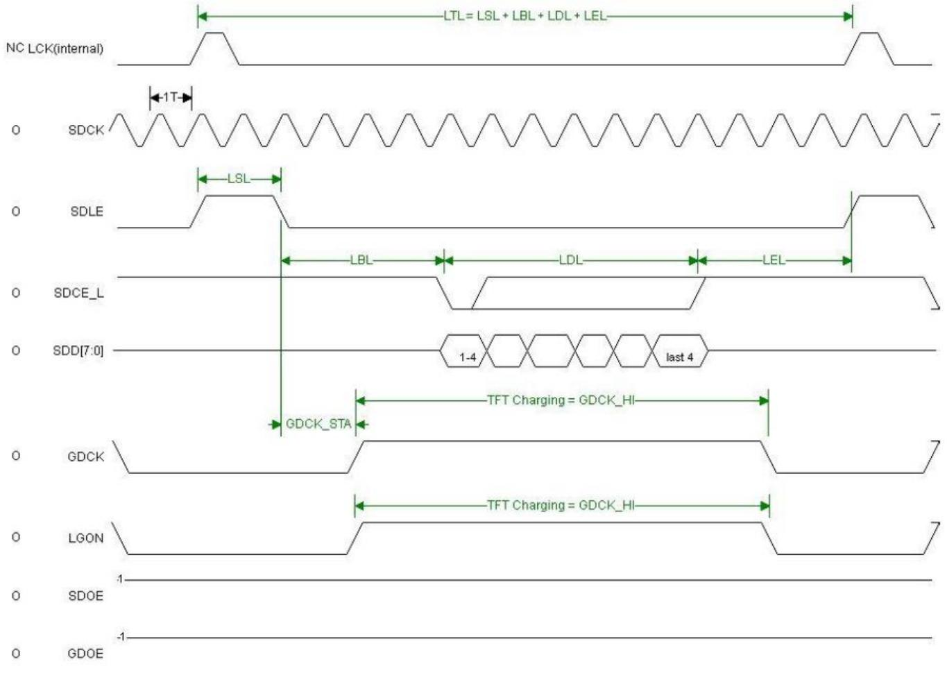
Figure 1 Line Timing in Mode 3
