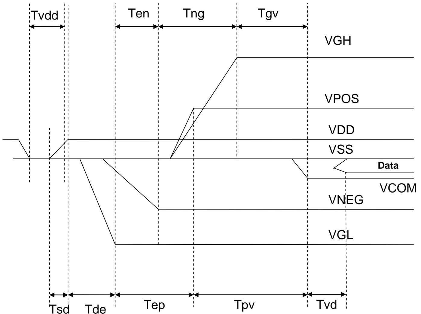
Note: If move from standby mode or power down to power on, VDD voltage must be set GND in the period of 700ms before VDD power on.
