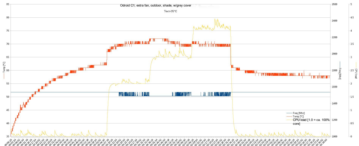
Odroid C1, extra fan, outdoor, shade T=35°C, IOT.ZPSET1510.1 kit (light grey)
