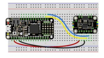
Board 3V to sensor VIN (red wire)
