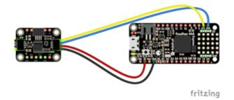
Board 3V to sensor VIN (red wire)
