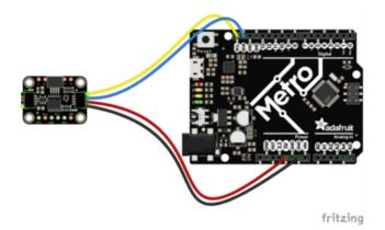
Board 5V to sensor VIN (red wire)
