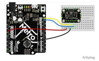
Board 5V to sensor VIN (red wire)
