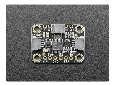
For the screens that have 1mm pitch FPC cables, you can plug the cable right into the connector. The majority of medium/large touchscreens have that kind of connector. If you have another kind of touch screen, the four X/Y contacts are available on 0.1" pitch breakouts so you can hand-solder or wire them.
