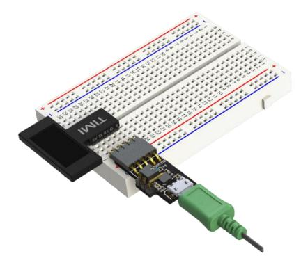
The BBM Programmer can also be directly connected to the appropriate row of 5 male pins on BBM products such as TIMI-96 if direct programming is desired instead.
