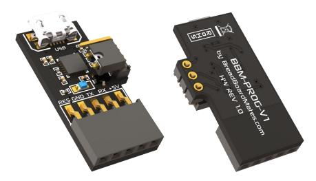
The BBM-PROG features a 3-pin jumper with shunt, which is present to change the way the programmer handles the Reset line, utilised by TIMI and other devices.
