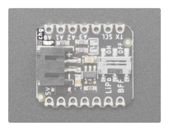
The charge LED, located in the upper left corner of the board, lights up when the battery is charging. Charging occurs only when the QT Py is plugged into USB power.
