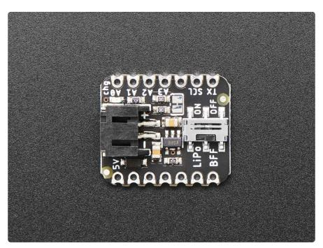
This little lipo charger is designed to fit onto the back of any QT Py board, and make it easy for portable powering. Simply plug any standard 3.7V/4.2V lithium polymer or lithium-ion rechargeable battery into the JST plug on the end. When powered by the
