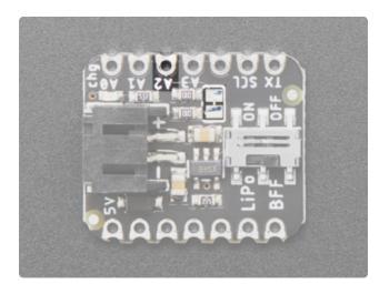
Pin A2, located to the left of center along the top edge of the board, is connected to the simple voltage divider, which will let your firmware detect basic modes. It measure the 5V line which is after a schottkey diode. If the voltage is over 4.0V, it is probably plugged into USB. If the voltage is 3.9V or below, its probably running on the Lipoly battery and you can roughly determine the battery state.
