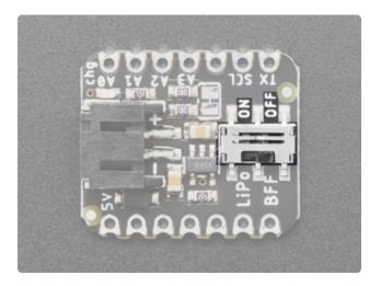
The power slide switch, located in the middle of the right side of the board, turns the BFF on or off, but only when the QT Py is NOT plugged into USB power.
