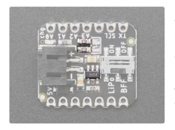
The MCP73831 lipo charge chip, located near the center of the board, will charge up the battery at 200mA max rate.
