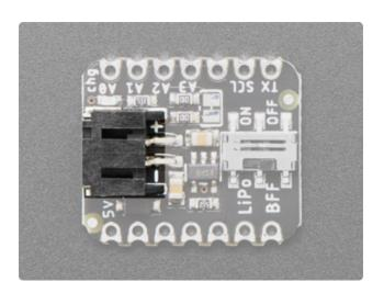
The battery JST connector, located in the middle of the left side of the board, enables you to plug in any standard 3.7V/4.2V lithium polymer or lithium-ion rechargeable battery to the BFF.
