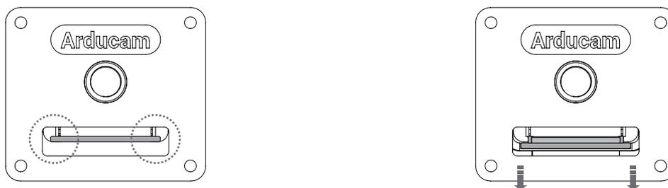
2. Insert the ribbon cable with pins facing away from the catch.
