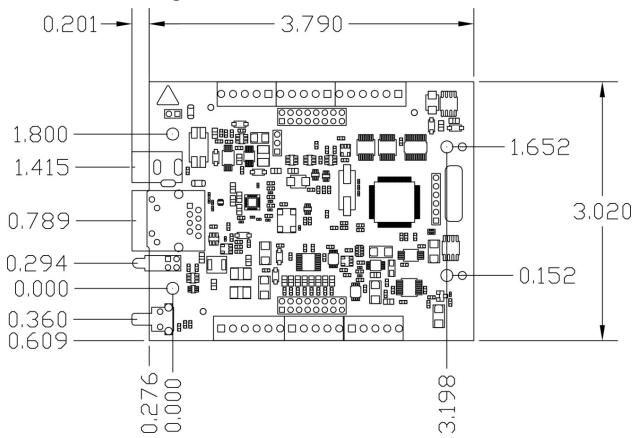
Figure 8. E-1608 device circuit board dimensions
