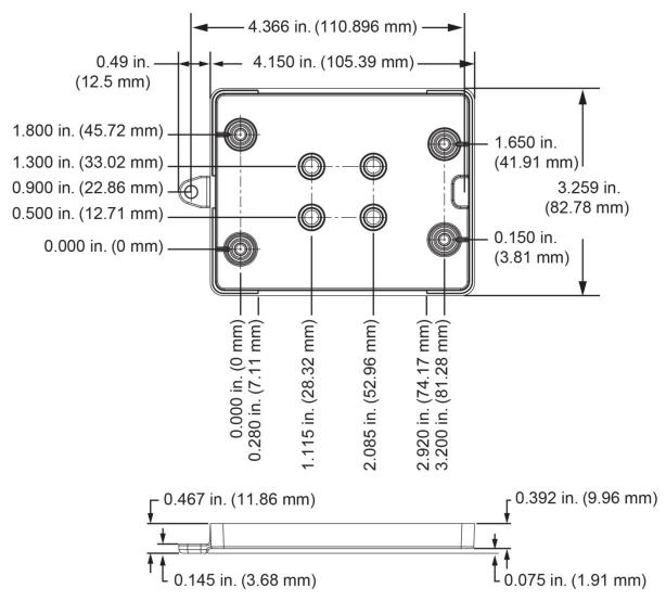
Figure 9. E-1608 bottom enclosure dimensions
