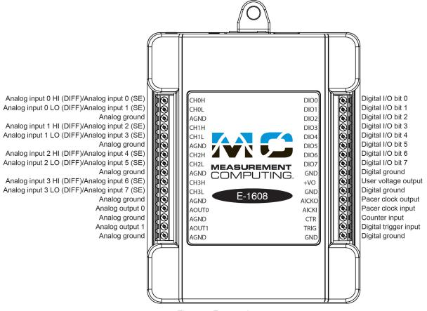
Figure 2. E-1608 pinout
