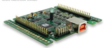
The USB-1608FS-Plus-OEM has the same specifications as the USB-1608FS-Plus, but comes in a board-only form factor with header connectors instead of screw terminals.
