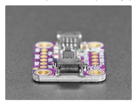
As with all Adafruit breakouts, we've done the work to make this handy accelerometer super easy to use. We've put it on a breakout board with the required support circuitry and connectors to make it easy to work with. Since I2C is supported, we've added SparkFun Qwiic (https://adafru.it/Fpw) compatible STEMMA QT (https://
