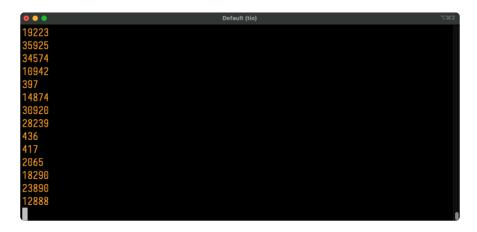
What do these values mean? In CircuitPython ADC values are put into the range of 16-bit unsigned values. This means the possible values you'll read from the ADC fall within the range of 0 to 65535 (or 2^16 - 1). When you twist the potentiometer knob to be near ground, or as far to the left as possible, you see a value close to zero.
