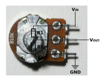
Connect one outside pin to ground Connect the other outside pin to voltage in (e.g. 3.3V)
