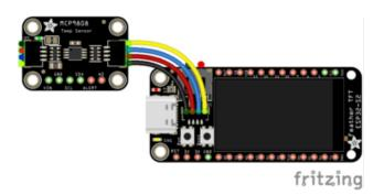
Using a STEMMA QT cable (https://adafru.it/Tff), connect the STEMMA QT connector on the MCP9808 to the STEMMA QT connector on the Feather.
