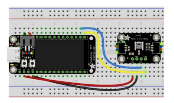
Make the following connections between the ESP32-S2 TFT Feather and the AHT20:
