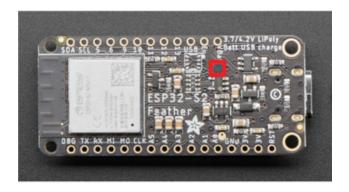
The LC709203 battery monitor (highlighted in red) is located on the bottom of the board near the VBAT pin label. Its I2C address is 0x0B. (0xb, which is returned by I2C scan, is the same as 0x0B, which simply has leading zeros.)
