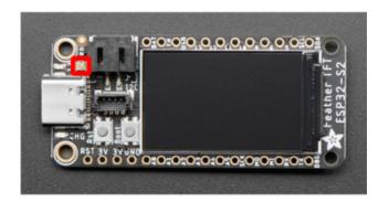
The NeoPixel (highlighted in red in the first image) is located above the USB C connector, next to the JST battery connector.
