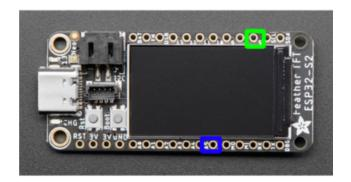
The A5 pin (highlighted in blue) is located along the bottom edge of the board, between A4 and SCK. It is labeled A5 on the silk.
