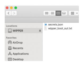
The BOOT drive will disappear and a new drive called WIPPER will appear with two files, secrets.json and wipper\_boot\_out.txt, on the filesystem.
