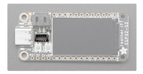
This JST SH 4-pin <u>STEMMA QT</u> (https://adafru.it/Ft4) connector breaks out I2C (SCL, SDA, 3.3V, GND). It allows you to connect to <u>various breakouts and sensors with STEM MA QT connectors</u> (https://adafru.it/Qgf) or to other things using <u>assorted associated accessories</u> (https://adafru.it/Ft6). It works great with any STEMMA QT or Qwiic sensor/device. You can also use it with Grove I2C devices thanks to <u>this handy cable</u> (https://adafru.it/Ndk).
