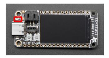
The red LED is located on the left side of the board, above the USB connector.
