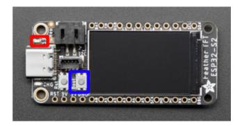
The red LED is located above the USB C connector, below the mounting hole, on the left end of the board.
