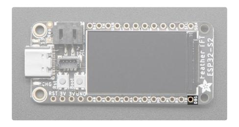
This is the Debug TX (DBG) pin. This is the hardware UART debug pin. You can connect this to a USB console cable in order to read the debug output from the ESP32 IDF (https://adafru.it/dDd). This is useful if you are writing software and need to see the low level debug output.
