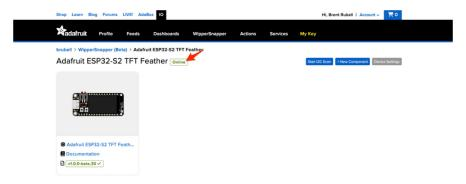
If the Feather appears offline on the website but was previously connected, press the Reset (RST) button to force the board to reboot.
