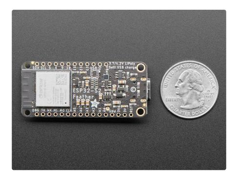
The ESP32-S2 is a highly-integrated, low-power, 2.4 GHz Wi-Fi System-on-Chip (SoC) solution that now has built-in native USB as well as some other interesting new technologies like Time of Flight distance measurements. With its state-of-the-art power and RF performance, this SoC is an ideal choice for a wide variety of application scenarios relating to the <a href="Internet of Things">Internet of Things</a> (IoT) (https://adafru.it/Bwq), <a href="weight: weight: wei
