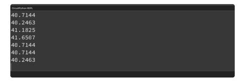
The CPU temperature in Celsius is printed out to the serial console!
