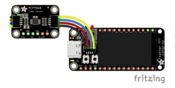
Simply connect the STEMMA QT cable from the STEMMA QT port on your board to the STEMMA QT port on the MCP9808.
