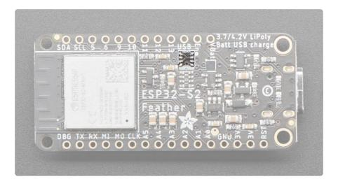
The ESP32-S2 TFT Feather comes with an unpopulated space for a BME280 Temperature, Humidity and Barometric Pressure Sensor.
