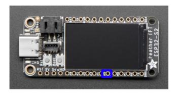
The D5 pin (highlighted in blue) is located along the bottom edge of the board, between A4 and SCK. It is labeled A5 on the silk (the pin has multiple name options).
