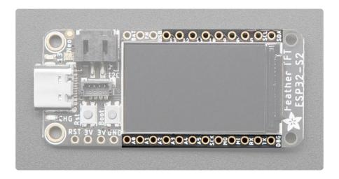
These are the logic pins that can be used to connect FeatherWings, sensors, servos, LEDs and more!
