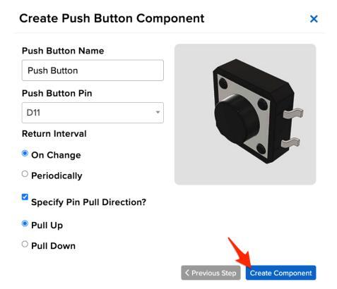
WipperSnapper should send a command to your board, telling it to configure the GPIO pin you selected to behave as a digital input pin and to enable it to pull up the internal resistor. Your WipperSnapper dashboard should also show the new push button component.
