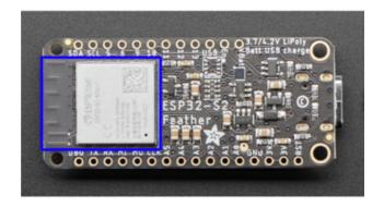
The ESP32-S2 microcontroller (higlighted in blue) is located on the bottom of the board, opposite the USB C connector.
