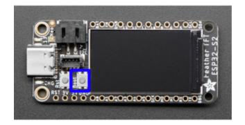
The boot button (highlighted in blue) is between the reset button and the TFT display. It is labeled Boot on the silk.
