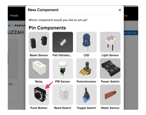
The next screen presents you with options for configuring the push button. Start by selecting the Feather's digital pin you connected to the push button.
