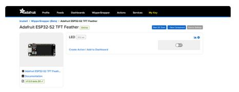
On the device interface, toggle the LED component by clicking the toggle switch. This should turn your Feather's built-in LED on or off.
