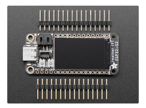
The color TFT is connected to the SPI pins, and uses additional pins for control that are not exposed to the breakout pads. It's the same display as you see here, with 240x135 pixels and is IPS (https://adafru.it/XLA) so you get bright color at any angle. The backlight is also connected to a separate pin so you can PWM the backlight up and down as desired.
