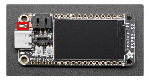
On the Feather TFT ESP32-S2, the red LED is on pin 13.
