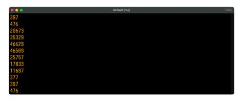
What do these values mean? In CircuitPython ADC values are put into the range of 16-bit unsigned values. This means the possible values you'll read from the ADC fall within the range of 0 to 65535 (or 2^16 - 1). When you twist the potentiometer knob to be near ground, or as far to the left as possible, you see a value close to zero.
